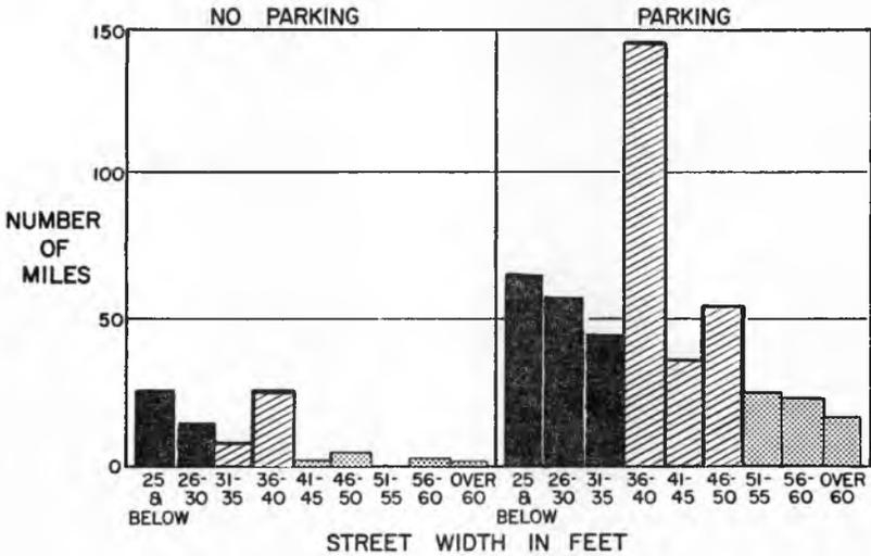
Fig. 19. Parking facilities on urban state system by street width.
