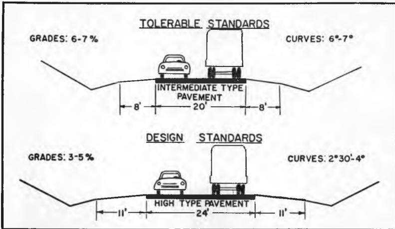
Fig. 11. Comparison of standards for primary highways.
