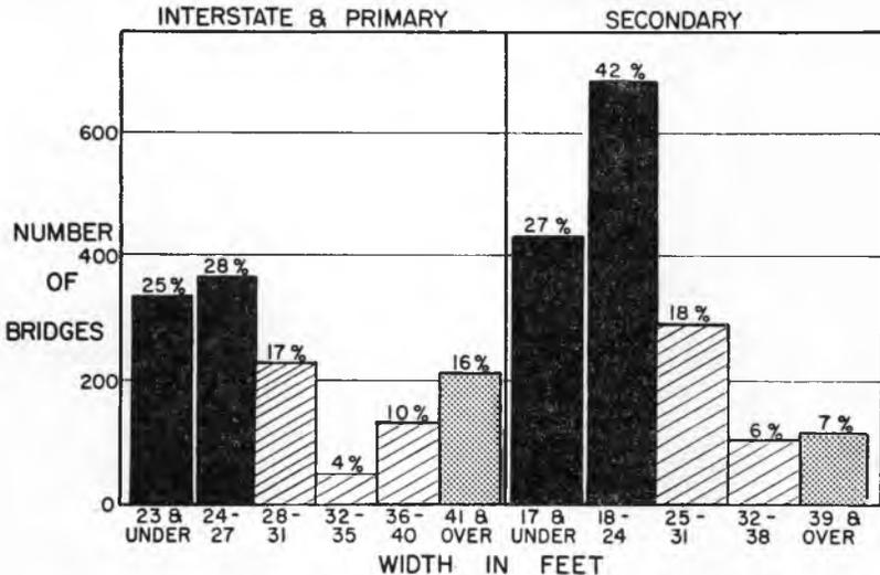
Fig. 15. Bridge widths on 2-lane rural highways.
