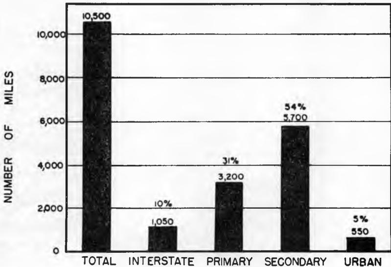
Fig. 6. Classification of the state highway system.
