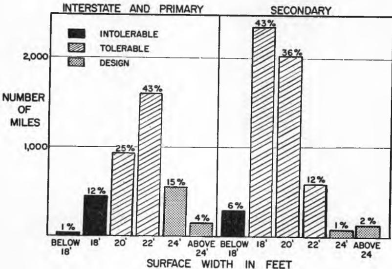
Fig. 12. Surface widths on 2-lane rural highways.
