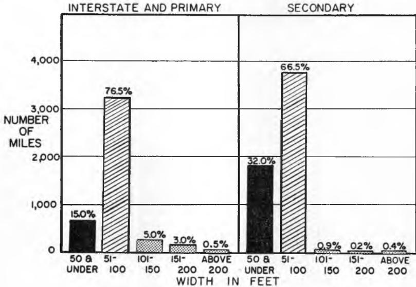
Fig. 14. Right of way widths on rural state system.
