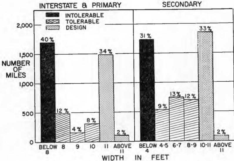
Fig. 13. Shoulder widths on rural state system.
