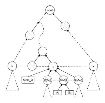
Figure 4. Hash tree for  $\alpha$ -correctness. The shaded nodes forms the authentication path of data item  $A_i^i$
