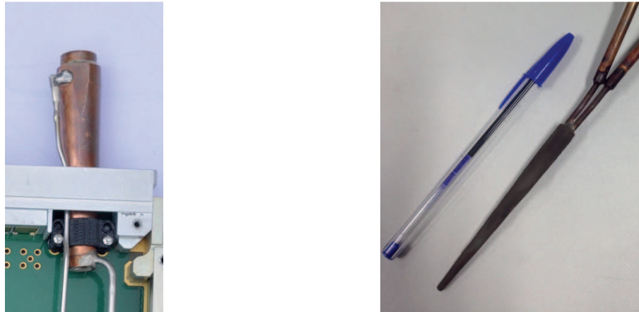
Figure 3: Pictures of the tested LHP condenser (left-hand side) and mini-VCS plug evaporator (right-hand side).
