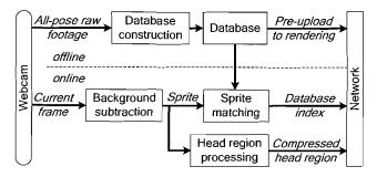
Figure 2: Acquisition module
