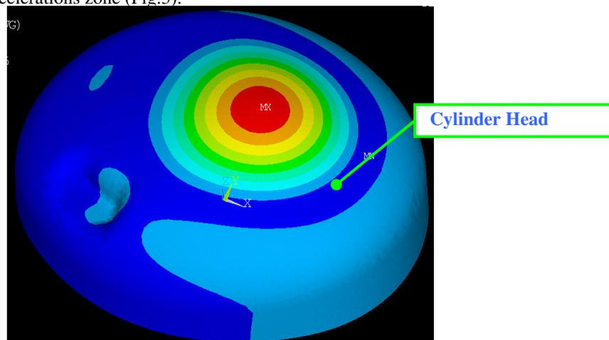
Figure 3: Upper shell's mode in the 3150 Hz third octave band
