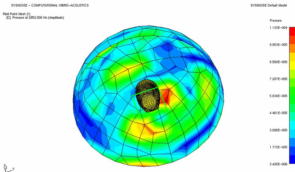
Figure 6: External pressure distribution from the B.E.M. calculation at 2950 Hz
