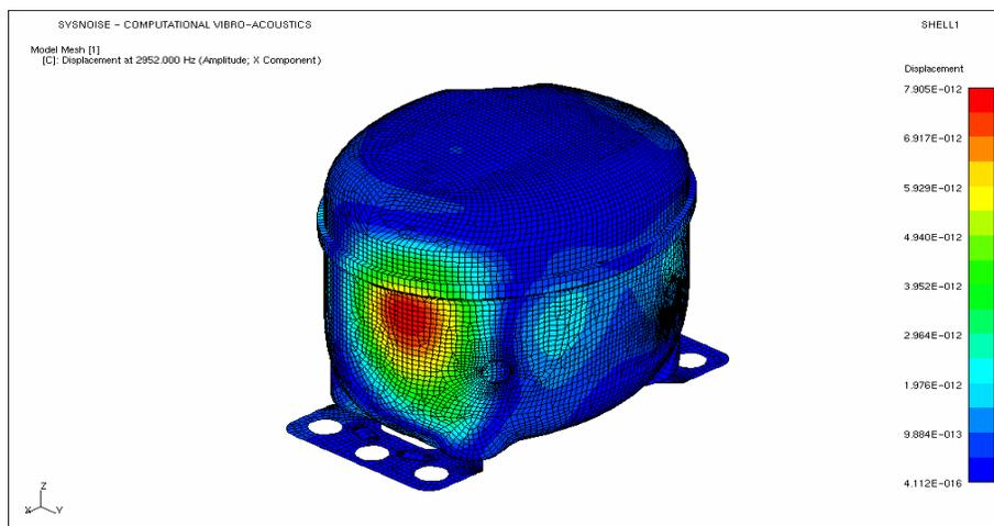
Figure 5: Forced cavity's pressure distribution at 2950 Hz
