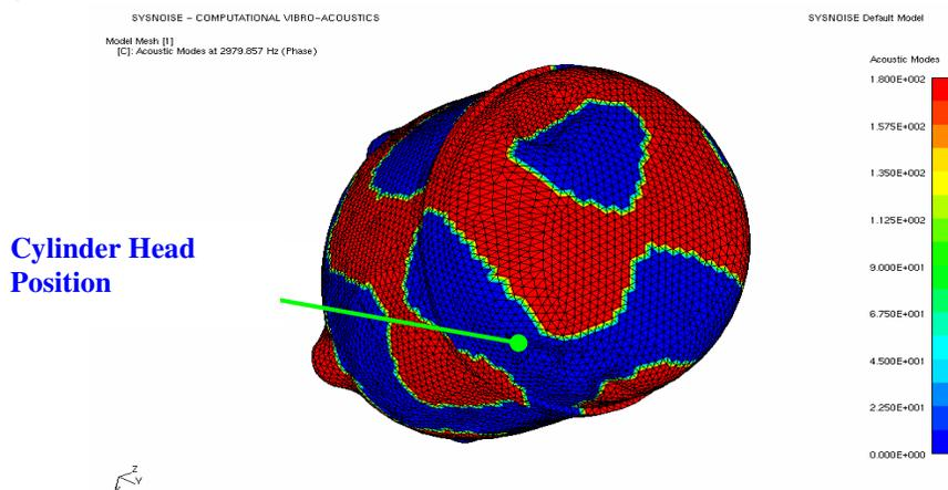
Figure 4: Cavity's pressure distribution at 2979 Hz (closest step to 2950 Hz)
