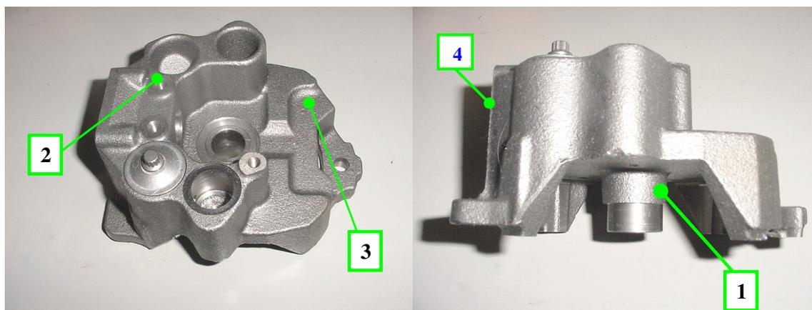
Figure 2: Some positions on the crankcase for accelerations measurement
