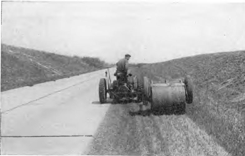
Berm roller. A manufactured roller, weight 500 to 1,500 pounds, depending on filler.
