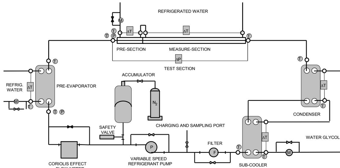
**Figure 1:** Schematic view of the experimental rig
