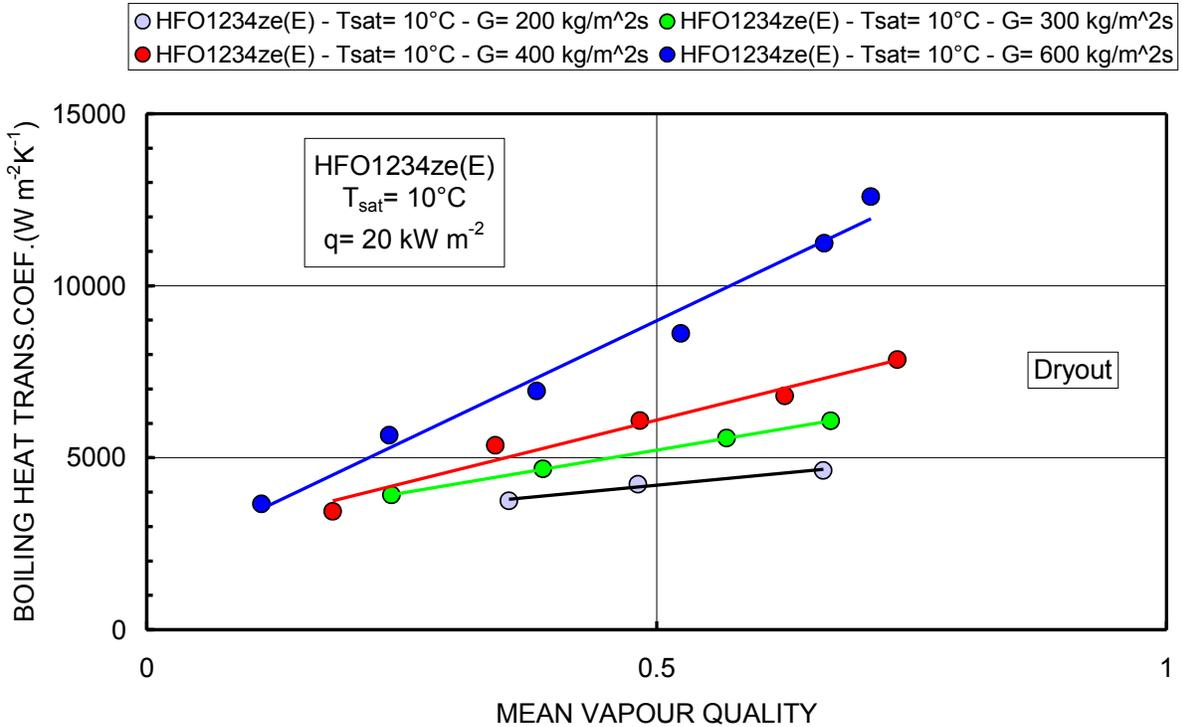
**Figure 3a:** Average heat transfer coefficient on refrigerant side vs. mean vapour quality and refrigerant mass flux at  $10^{\circ}C$  of saturation temperature and  $20 kW m^{-2}$  of heat flux for HFO1234ze(E)
