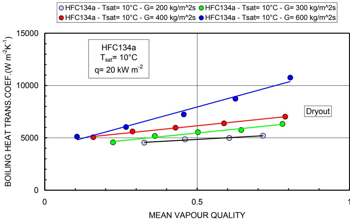
**Figure 3b:** Average heat transfer coefficient on refrigerant side vs. mean vapour quality and refrigerant mass flux at  $10^{\circ}C$  of saturation temperature and  $20 kW m^{-2}$  of heat flux for HFC134a
