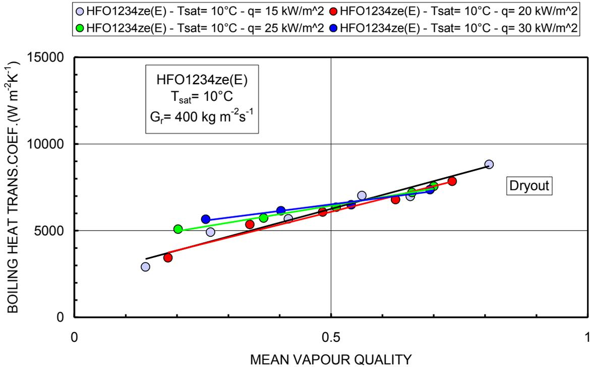
**Figure 4a:** Average heat transfer coefficient on refrigerant side vs. mean vapour quality and heat flux at 10°C of saturation temperature and 400 kg m<sup>-2</sup> s<sup>-1</sup> of refrigerant mass flux for HFO1234ze(E)
