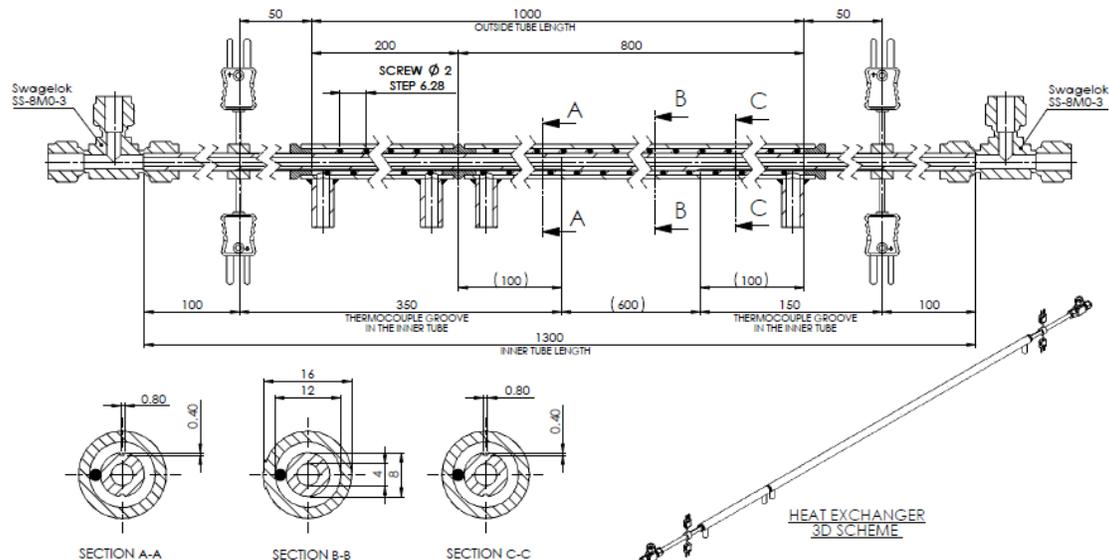
**Figure 2:** Schematic view of the test section
