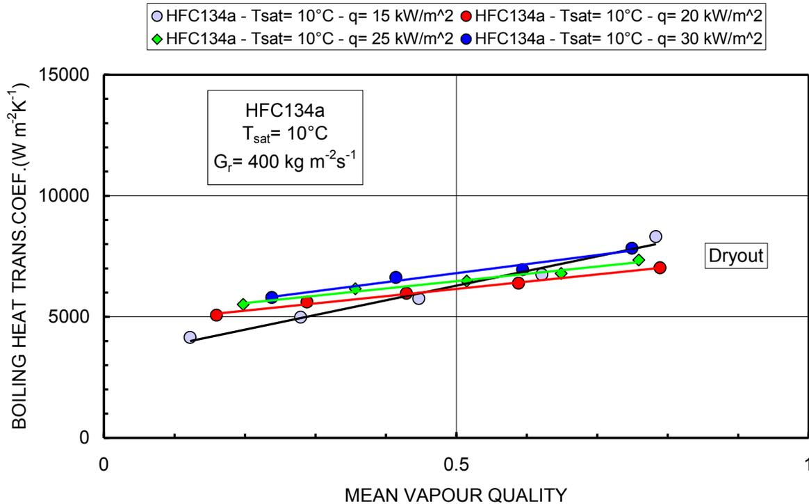
**Figure 4b:** Average heat transfer coefficient on refrigerant side vs. mean vapour quality and heat flux at 10°C of saturation temperature and 400 kg m<sup>-2</sup> s<sup>-1</sup> of refrigerant mass flux for HFC134a
