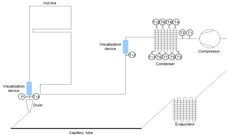
**Figure 1:** Schematic of the refrigerator experimental apparatus
