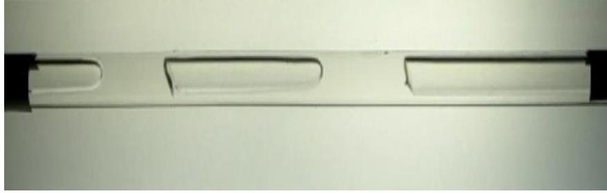
**Figure 6:** Phase behavior at the dryer inlet of the refrigeration cycle
