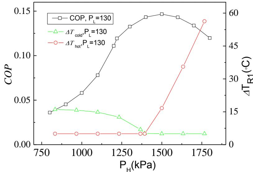
**Figure 4.** The variation of  $COP$ ,  $\Delta T_{hot}$ ,  $\Delta T_{cold}$  with the high pressure ( $z_{1,1}=0.2$ ,  $z_{1,3}=0.6$ ,  $P_L=130$ kPa)
