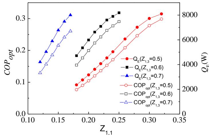
**Figure 6.** The variation of  $COP_{opt}$  and  $Q_E$  with the fraction of R23 ( $T_G=140\text{ }^{\circ}C$ ,  $T_H=20\text{ }^{\circ}C$ ,  $T_L=-50\text{ }^{\circ}C$ ,  $z_{3,3}=0.03$ )
