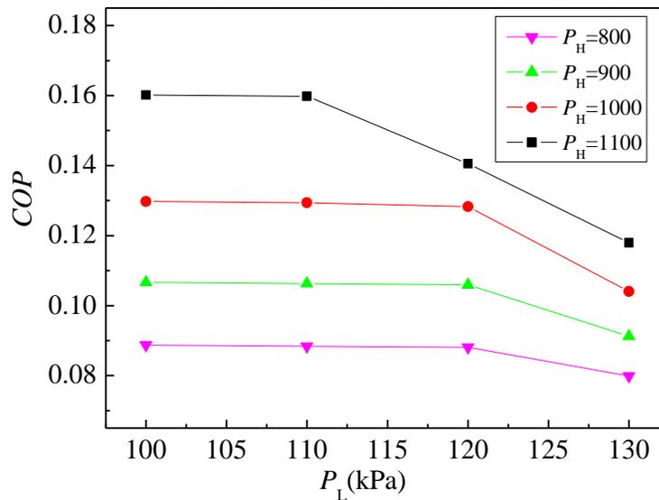
**Figure 3.** The variation of  $COP$  with the low pressure  $P_L$  ( $z_{1,1}=0.2, z_{1,3}=0.6$ )
