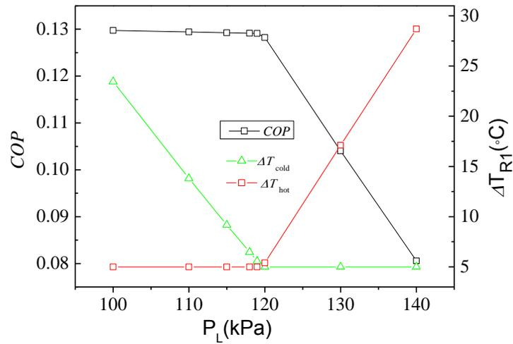
**Figure 5.** The variation of  $COP$ ,  $\Delta T_{hot}$ ,  $\Delta T_{cold}$  with the low pressure ( $z_{1,1}=0.2$ ,  $z_{1,3}=0.6$ ,  $P_H=1000\text{kPa}$ )
