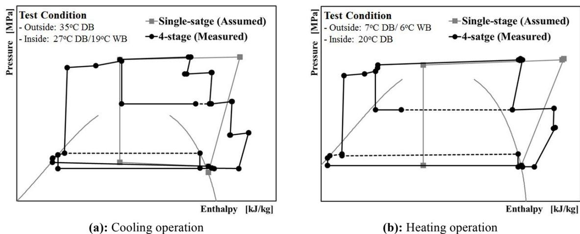
Figure 16: P-h diagram in each operating mode
