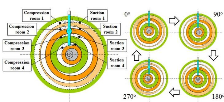
Figure 6: Operation mechanism
