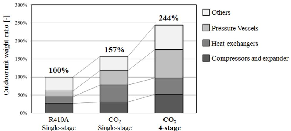
**Figure 18:** Outdoor unit weight at 10HP
