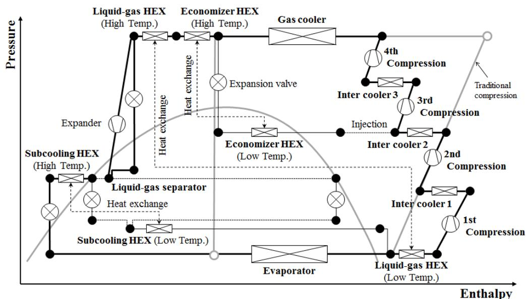
Figure 1: P-h diagram of high efficiency four-stage compression and cooling system
