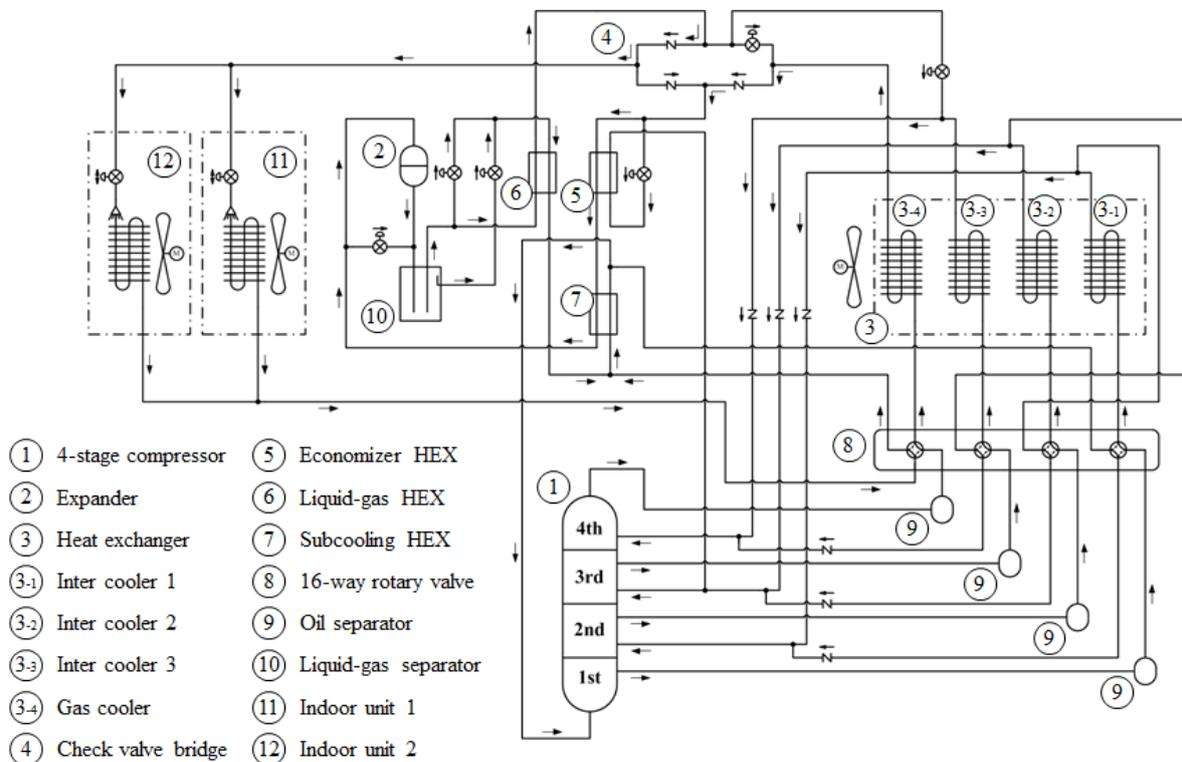
Figure 3: Refrigerant circuit of test system
