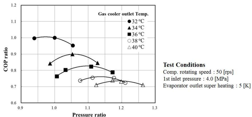
Figure 15: Cooling COP ratio in each outside temperature
