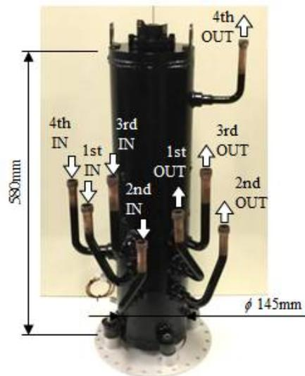
Figure 9: Four-stage compressor with one casing
