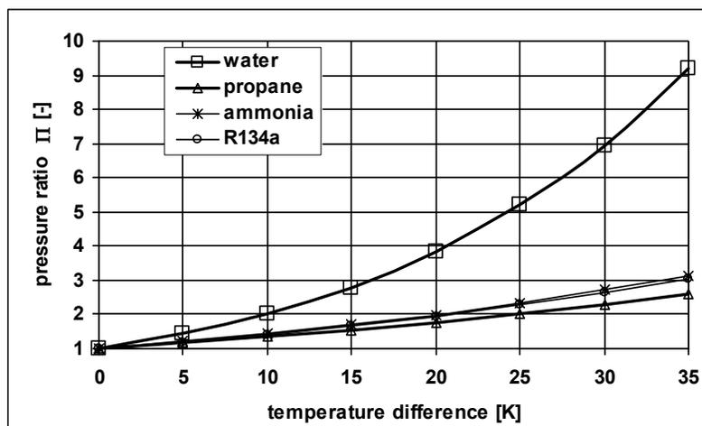
Figure 1: Pressure ratio as function of temperature lift
