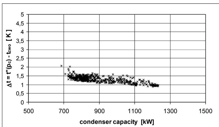
Figure 7: Temperature difference as a function of condenser capacity
