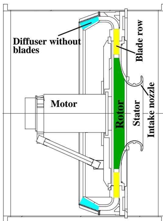
Figure 4: Compressor design scheme
