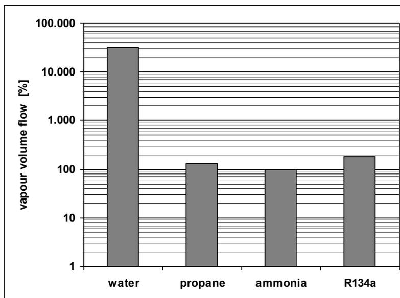
Figure 2: Comparison of volume flows at the same cooling capacity
