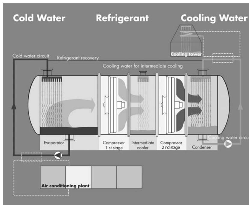
Figure 3: Design of an R718 turbo chiller
