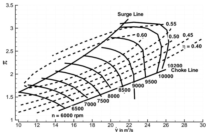
Figure 5: Compressor characteristics field with surge and choke line
