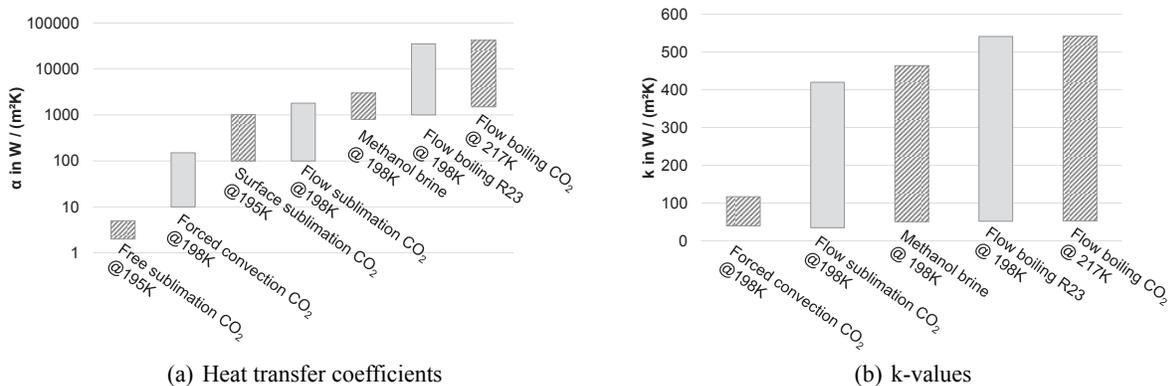
**Figure 3: Comparison of heat transfer coefficients for forced convection, sublimation and flow boiling.**
