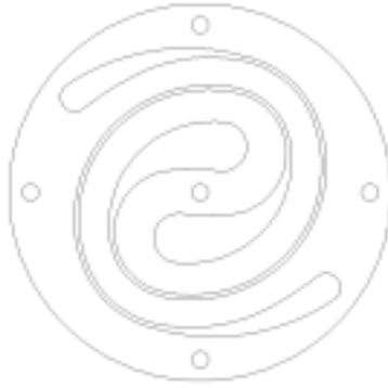
Figure 2. A typical planar spring.
