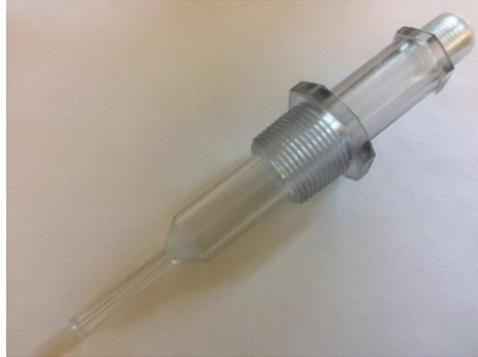
**Figure 6:** 3D printed transparent convergent-divergent nozzle
