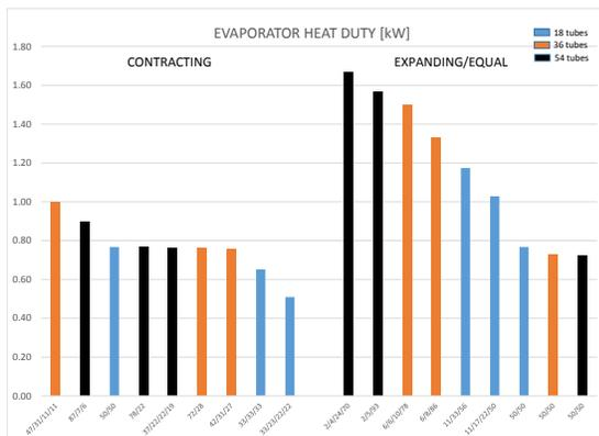
Figure 6: Best evaporator pass arrangements
