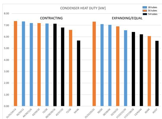
Figure 3: Best condenser pass arrangements
