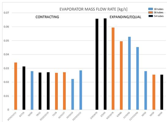
Figure 7: R410A mass flow rate for best evaporators
