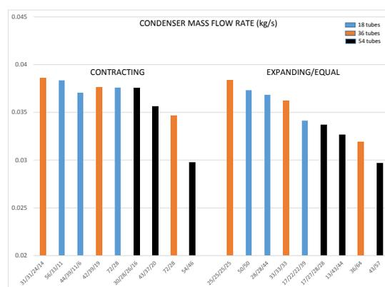
Figure 4: R410A mass flow rate through best condensers
