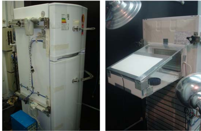
Figure 8: Door-opening device (left) and visualization improvement (right)
