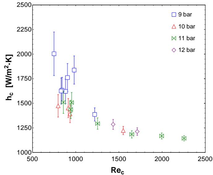
**Figure 5:** Experimental condensation heat transfer coefficients as a function of the condensate Reynolds number for a set of experiments carried out for a constant superheating degree of 20°C and different condensation pressures
