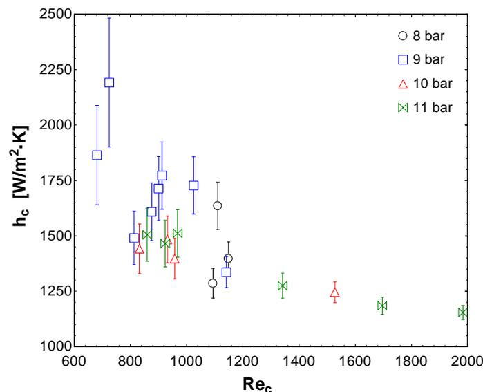
**Figure 4:** Experimental condensation heat transfer coefficients as a function of the condensate Reynolds number for a set of experiments carried out for a constant superheating degree of 10°C and different condensation pressures
