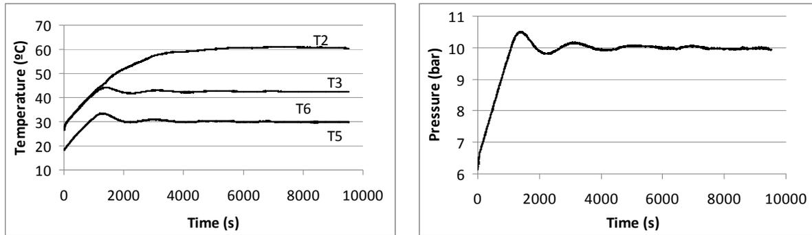
**Figure 3:** Experimental measured values of the refrigerant and water temperatures at the inlet and outlet of the condenser and the condenser pressure for a characteristic test run
