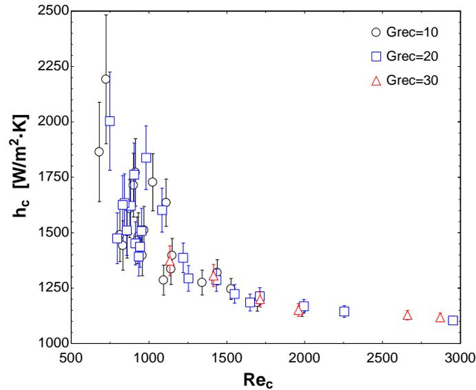
**Figure 6:** Experimental condensation heat transfer coefficients as a function of the condensate Reynolds number for a set of experiments carried out with superheating degrees of 10°C, 20°C and 30°C
