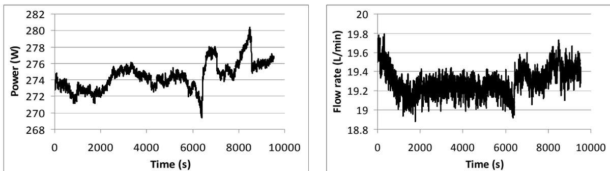
**Figure 2:** Experimental values of the power supplied to the heating cable in the evaporator and the water flow rate through the condenser
