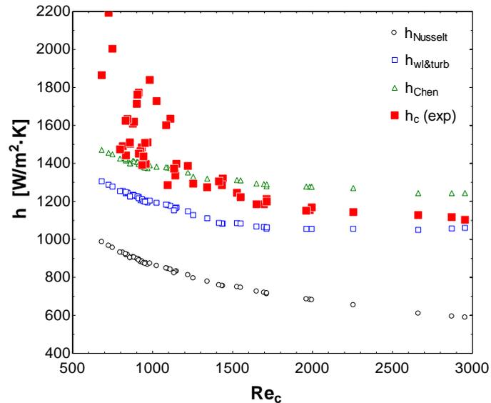
**Figure 7:** Experimental values of the condensation heat transfer coefficient as a function of the condensate Reynolds number and predicted values from different correlations
