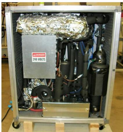
**Figure 2:** Heat pump components housed within unit
