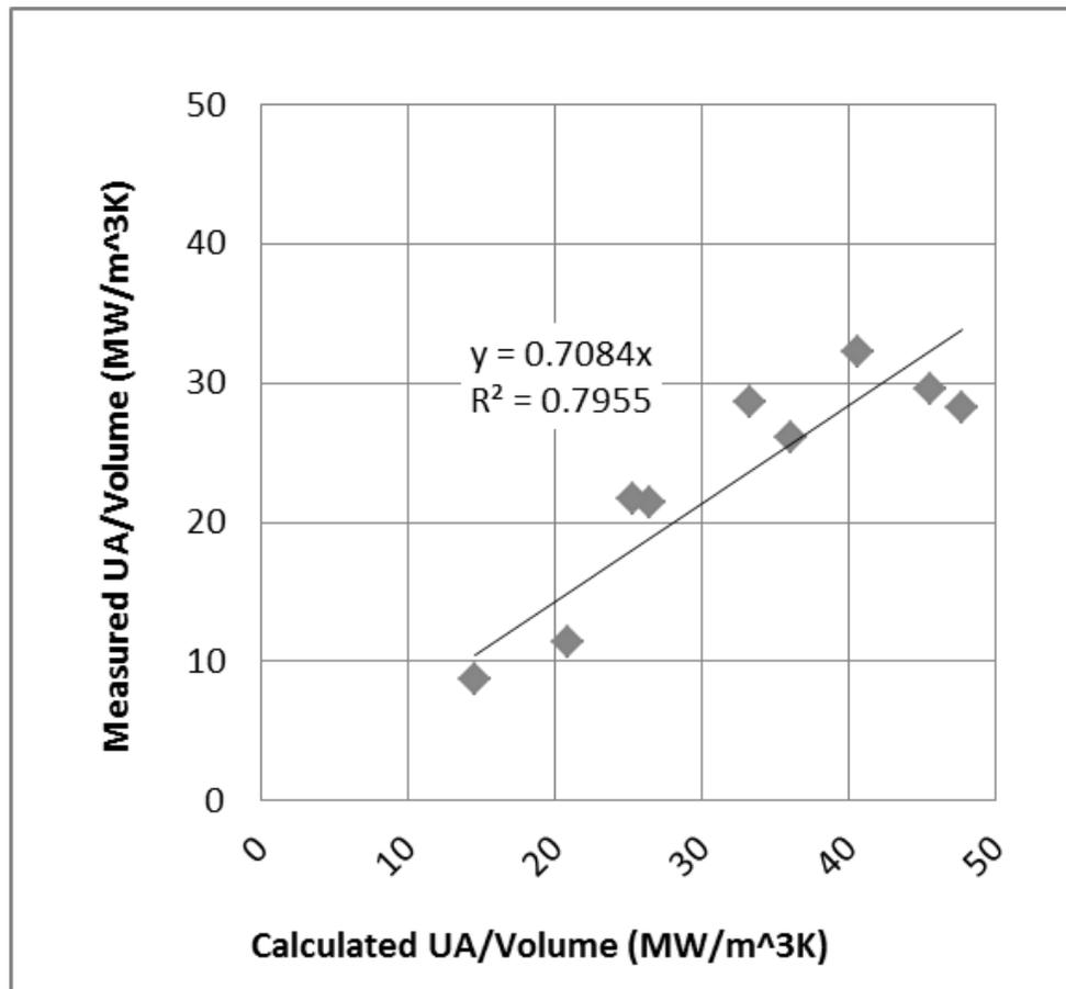
**Figure 4:** Fit of measured values to equation 12 predictions.
