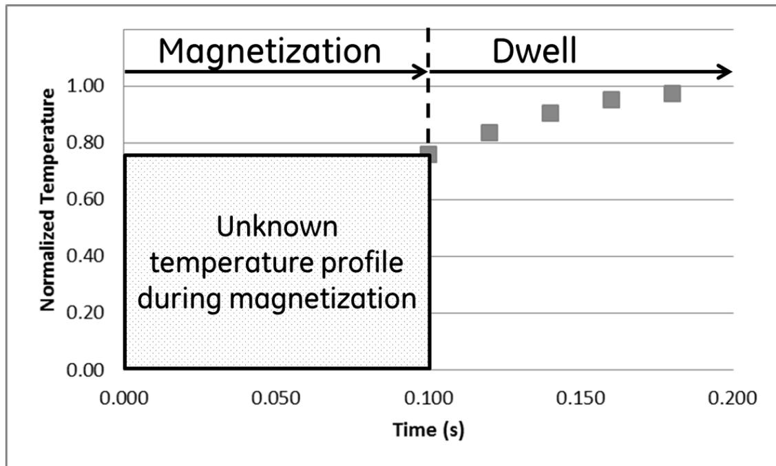
**Figure 3:** Example of measured temperature with respect to dwell time.
