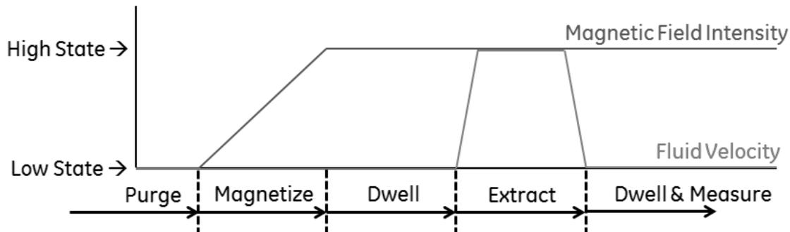
Figure 1: Test profiles for magnetic field and fluid velocity.
