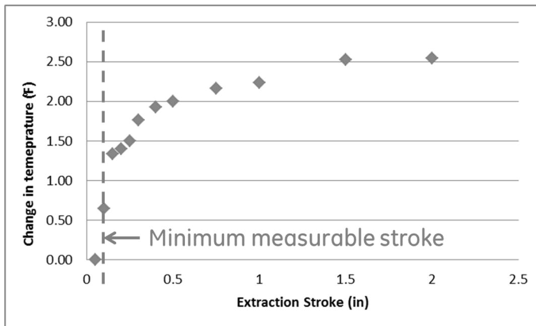
**Figure 2:** System thermal response for various stroke lengths with constant fluid temperature.
