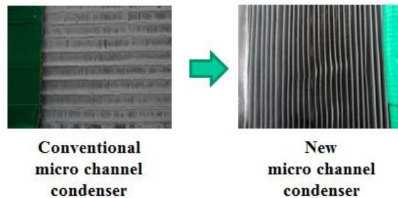
**Figure 8:** State of the frost after 30 minutes (air side velocity 1.5m/s, temp. 2/1 °C)
