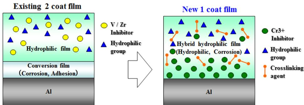
Figure 9: Development of new post coating system
