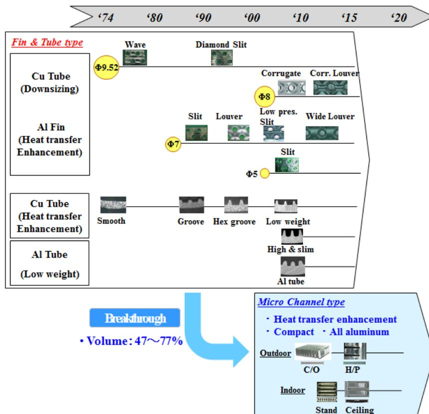
**Figure 1:** Trend of High Performance Heat Exchanger in Samsung
