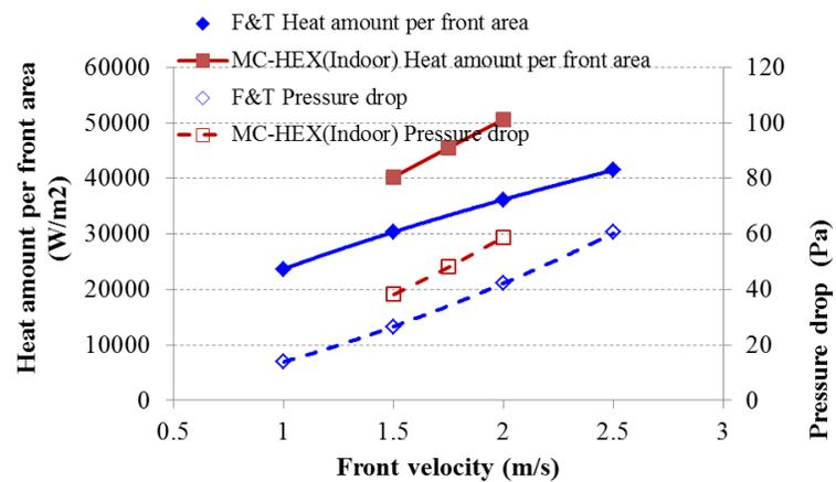
(b) About parallel flow heat exchanger for indoor unit (Condensation condition)
