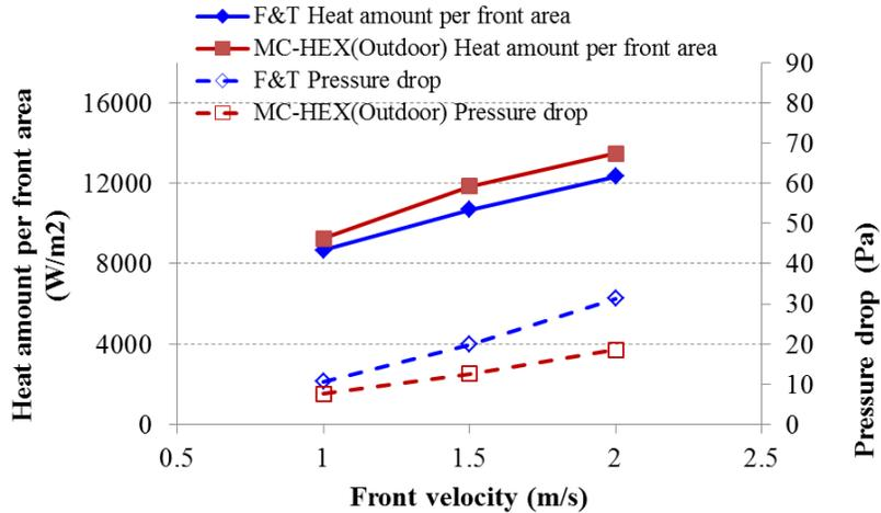
(a) About parallel flow heat exchanger for outdoor unit (Evaporation condition)
