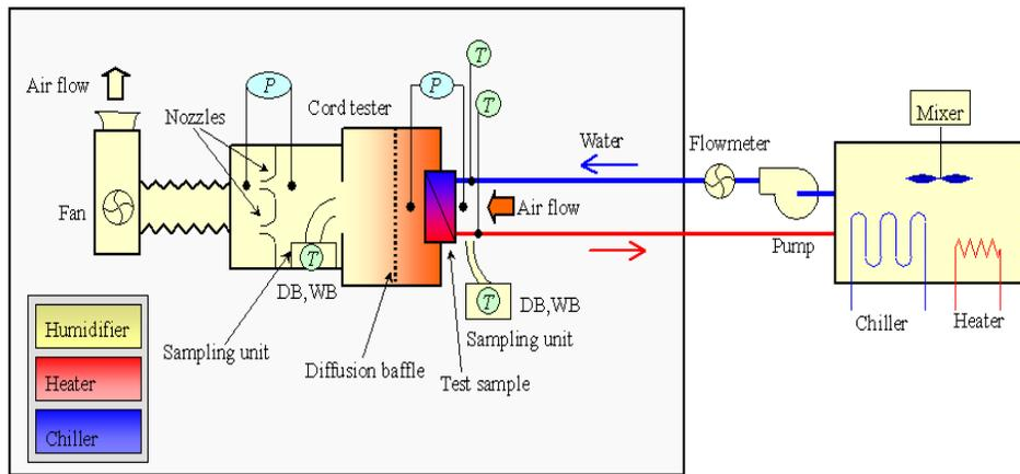
Figure 3: Schematic diagram of heat exchanger capacity test
