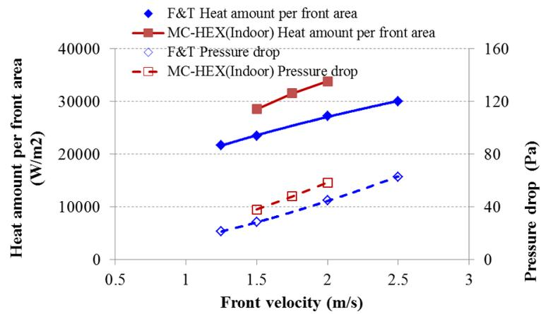
(a) About parallel flow heat exchanger for indoor unit (Evaporation condition)
