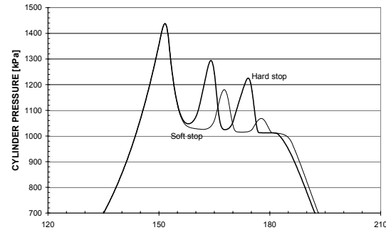
Figure 15: Effect of oil on hard and soft stop
