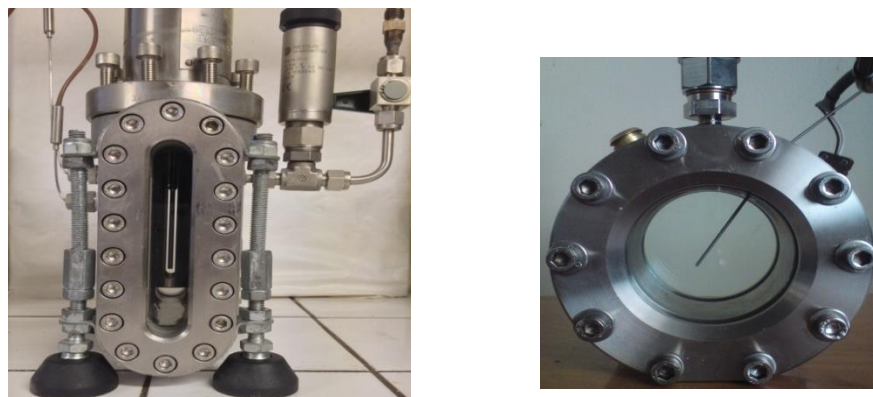
Figure 2: Viscosity/solubility/miscibility cell (left) and miscibility/solubility cell (right)
