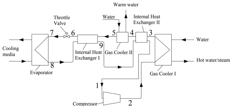
**Figure 4:** Proposed system schematic of CO<sub>2</sub> heat pump for dairy process
