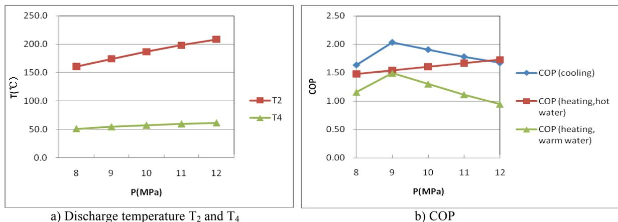
Figure 6: Simulation results and COP of the CO<sub>2</sub> heat pump
