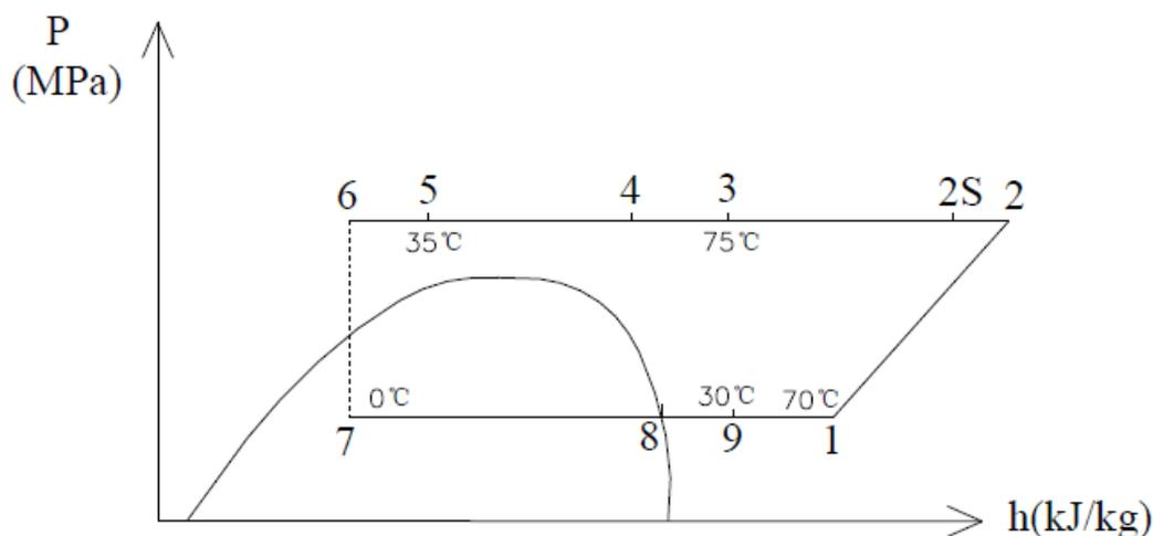
**Figure 5:** Pressure-enthalpy plots of CO<sub>2</sub> heat pump proposed for dairy process
