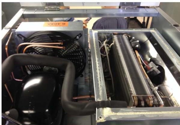
Figure 9: Top-mount refrigeration unit
