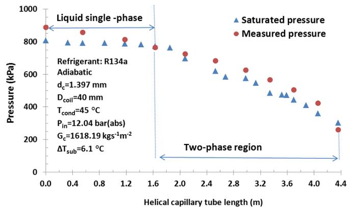
**Figure 6:** Saturation and measured pressure distribution through the adiabatic capillary tube with inlet temperature of 45°C
