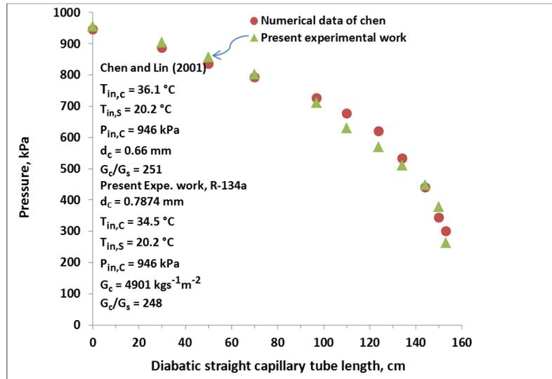
**Figure 7:** Comparison of the present experimental work and numerical results of Chen and Lin (2001), for R134a flow through non-adiabatic straight capillary tube
