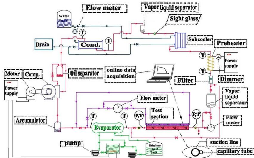
Figure 1: The schematic diagram of experimental set up
