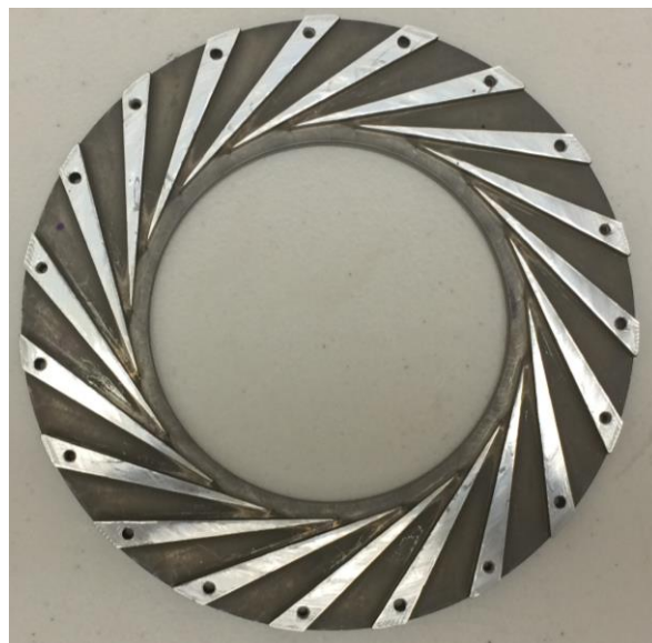
Figure 2: Fixed vane nozzle for 75 kW
