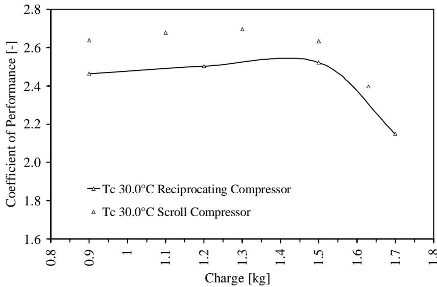
Figure 7: Coefficient of performance against system charge level
