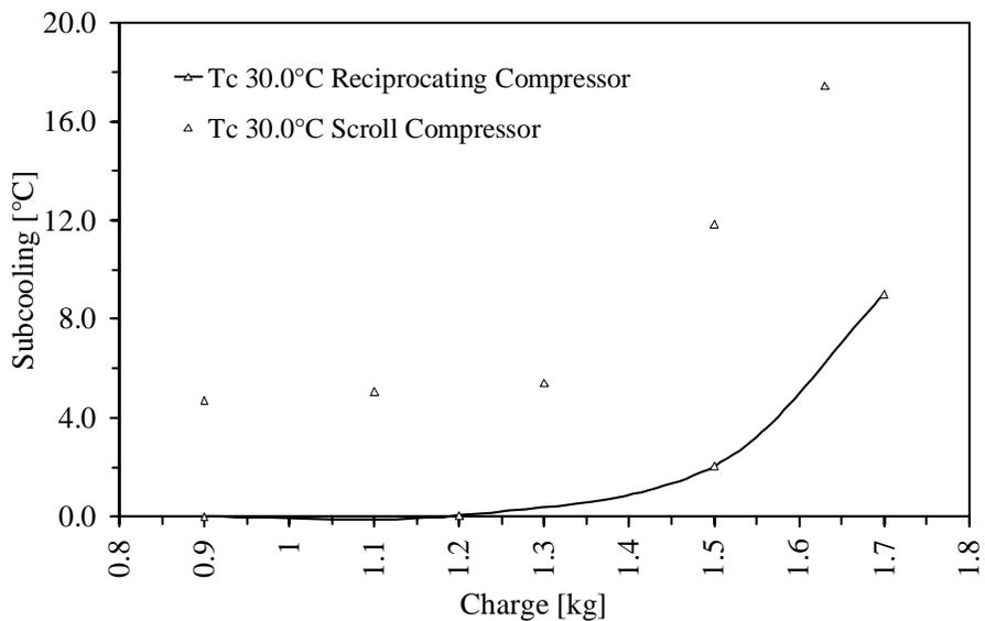
Figure 9: Subcooling against system charge level
