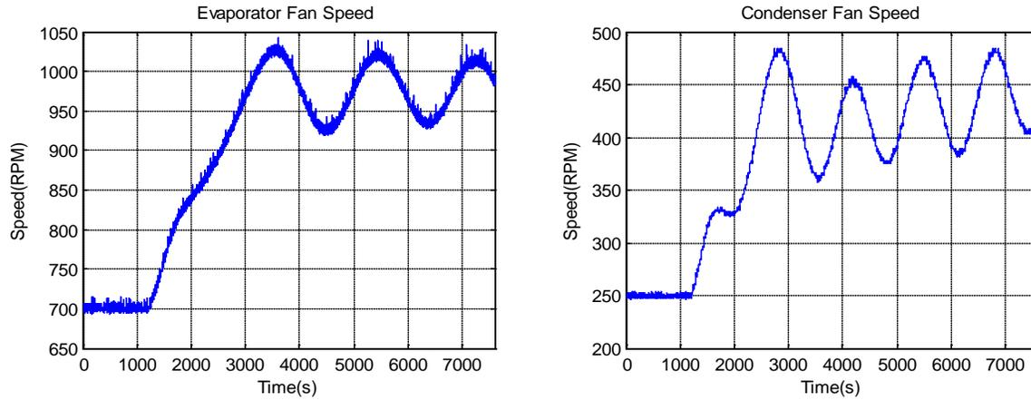
**Figure 10:** Evaporator and condenser fan speed
