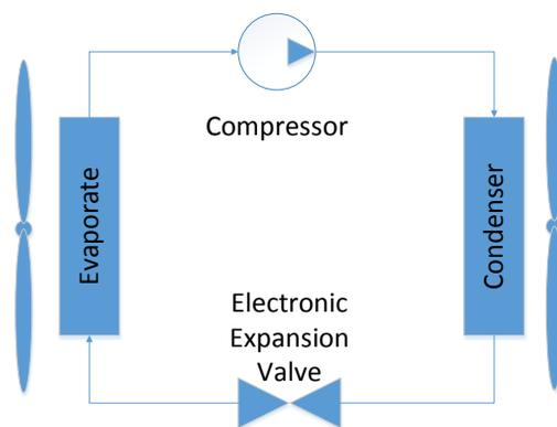
**Figure 1:** Diagram of a mini-split AC system
