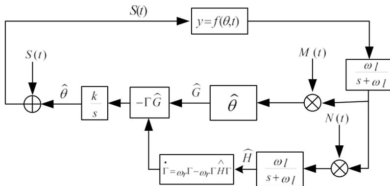
Figure 4: Diagram of Newton-based multi-variable ESC
