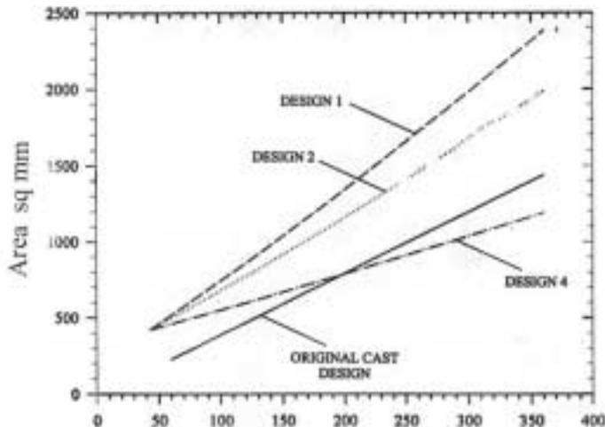
Fig.2 Volute area as a function of azimuth angle
