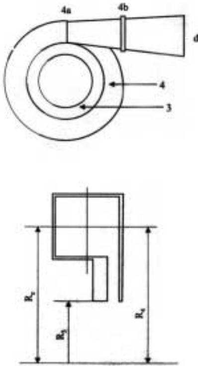
Fig.4 Compressor Diffusion System
