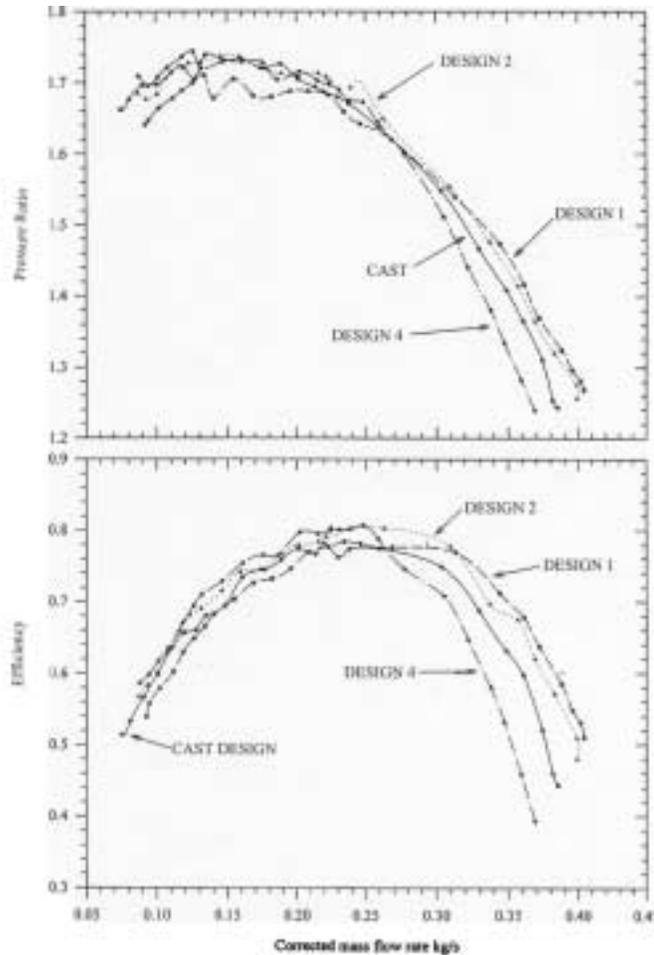
Figure 3. Effect of Volute Design on Compressor Stage Performance
