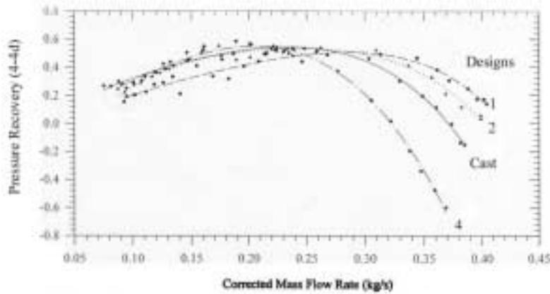
Fig.6c Volute Pressure Recovery (4-d) as a function of mass flow rate
