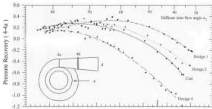
Fig.6a Pressure Recovery of Scroll (4-4a)
