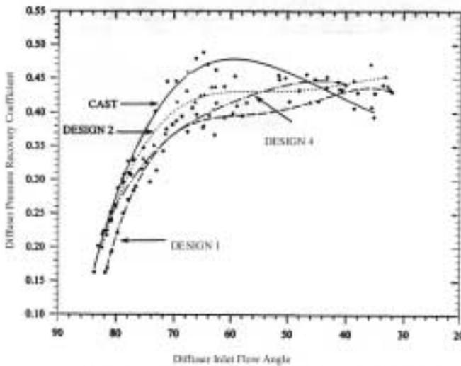
Fig.5 Variation of Diffuser Pressure Recovery Coefficient with Inlet Flow Angle
