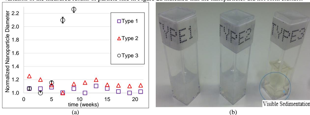
**Figure 2:** (a) Sedimentation test results for three types of nanolubricants and (b) visual observation of sedimentation for type 3 nanolubricant
