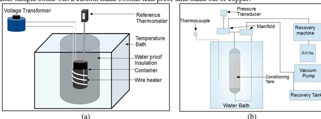
**Figure 1:** Experimental setups for measuring specific heat (a) and solubility (b) of nanolubricants
