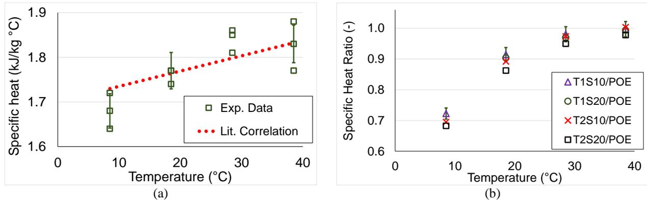
Figure 3: (a) Specific heat vs. temperature for POE oil and (b) Specific heat ratio vs. temperature for the nanolubricants
