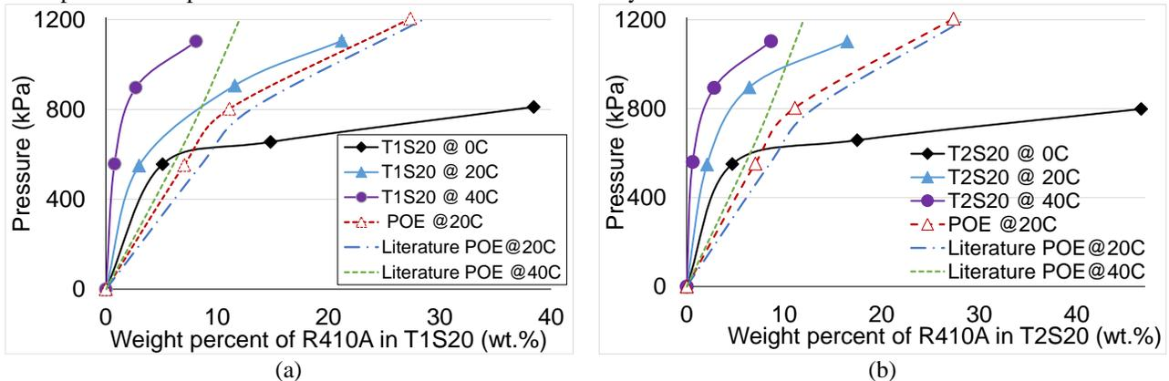
Figure 4: Pressure vs. refrigerant concentration in wt. % of R-410A in (a) T1S20 and in (b) T2S20 nanolubricants
