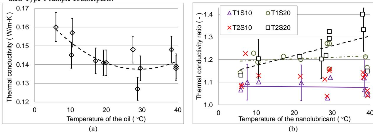
**Figure 5:** (a) Thermal conductivity vs. Temperature for POE oil and (b) Nanolubricant-POE thermal conductivity ratio
