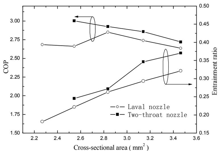
Figure 3: System COP and entrainment ratio of ejector with throat area of nozzle
