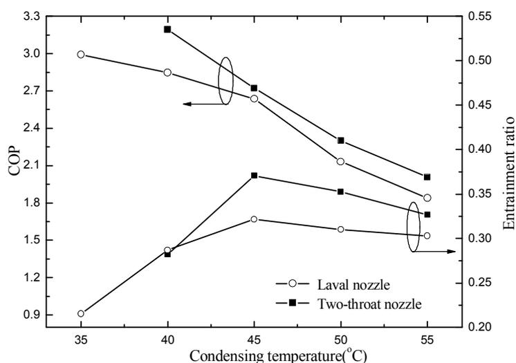
**Figure 4:** Variation of system COP and entrainment ratio of ejector with condensing temperature
