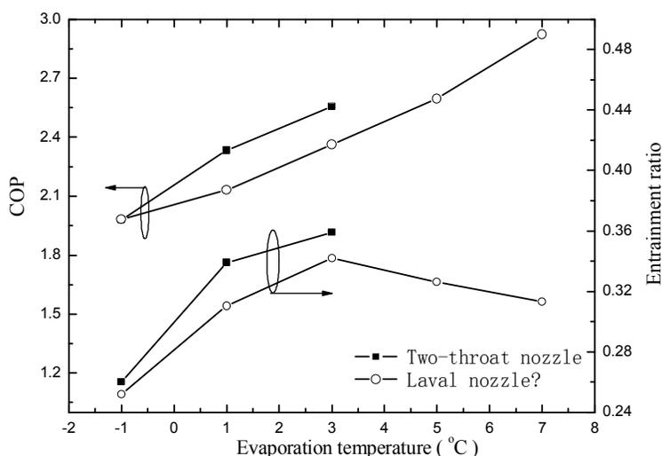
**Figure 5:** Variation of system COP and entrainment ratio of ejector with evaporation temperature
