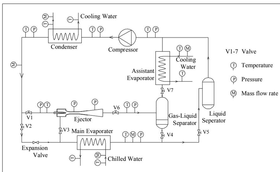
**Figure 1:** Diagram of experimental setup of TPERC System
