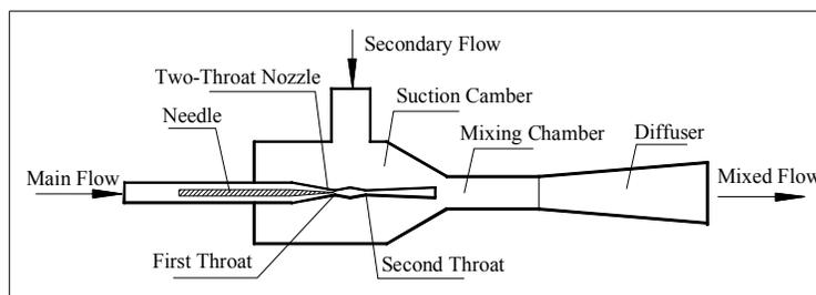
Figure 2: Schematic diagram of two-throat nozzle ejector
