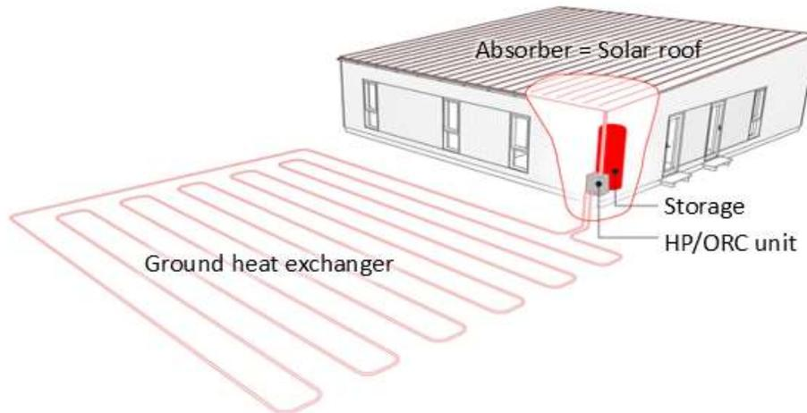
**Figure 1 :** HP/ORC reversible unit connected to a 120 m<sup>2</sup> solar roof and a horizontal ground heat exchanger (Innogie, 2012)
