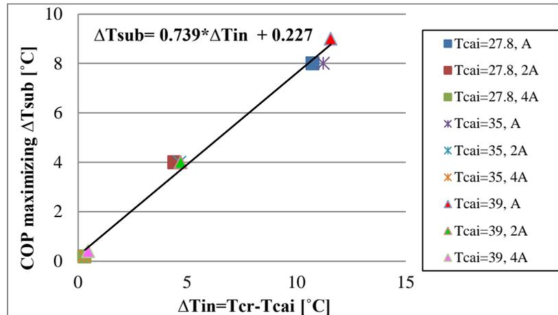
Figure 8: COP maximizing  $\Delta T_{sub}$  as a function of  $\Delta T_{in}$
