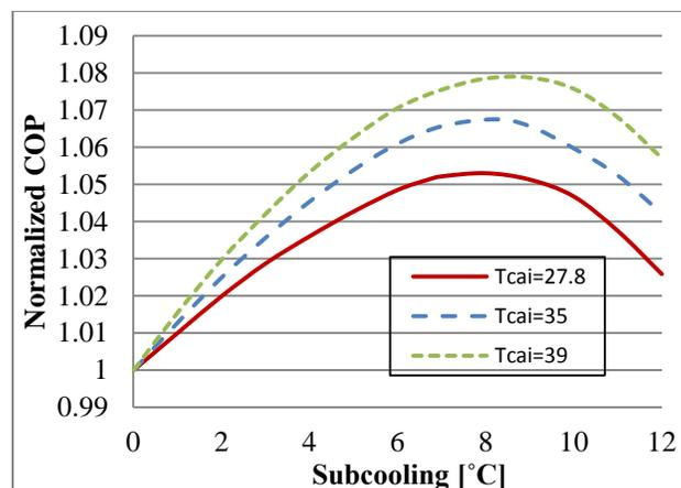
**Figure 5:** Effect of subcooling temperature on normalized COP (condition **A**, **B**, **C** in Table 3) for constant capacity
