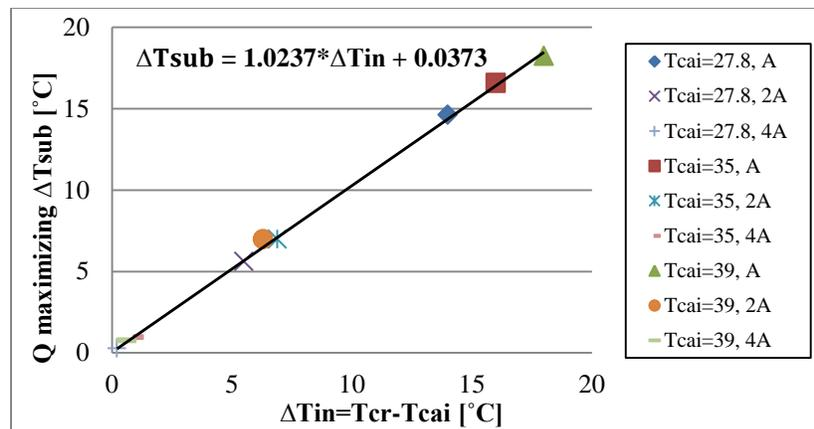
Figure 9: Q maximizing  $\Delta T_{sub}$  as a function of  $\Delta T_{in}$
