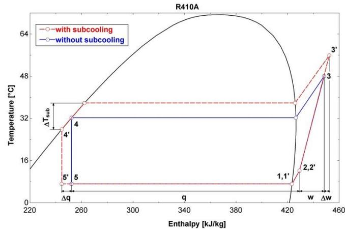
**Figure 1:** Temperature-specific enthalpy diagram of vapor-compression refrigeration cycle with/without subcooling
