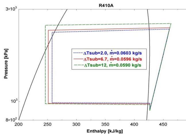
**Figure 4:** Effect of subcooling on refrigerant mass flow rates for  $\Delta T_{\text{sub}}=2.0^\circ\text{C}$ ,  $6.7^\circ\text{C}$ , and  $12^\circ\text{C}$
