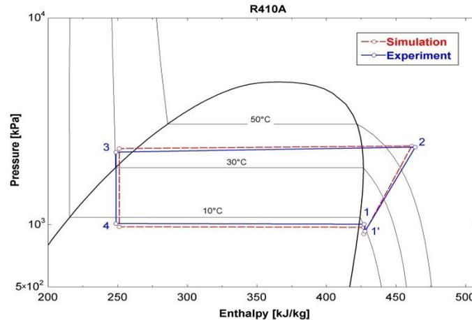
Figure 2: Pressure-specific enthalpy diagram (condition B in Table 3)
