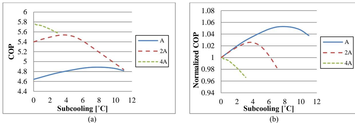
**Figure 6:** Effect of condenser size on subcooling improved COP presented in (a) actual and (b) normalized terms (condition **B** in Table 3)
