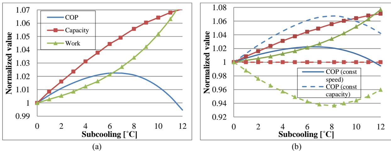
Figure 3: (a) Effect of subcooling temperature on normalized COP, cooling capacity, and compression work for constant compressor speed; (b) Comparison of subcooling effects on normalized COP, cooling capacity and compression work for constant compressor speed and constant cooling capacity (condition A in Table 3)
