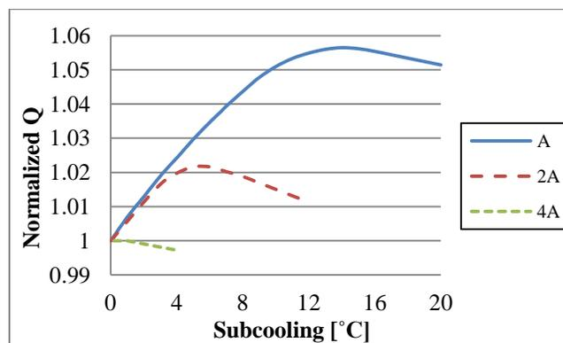
**Figure 7:** Effect of condenser size on subcooling improved cooling capacity  $Q$  presented in normalized way (condition **B** in Table 3)
