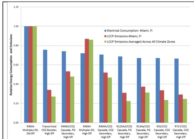
**Figure 3:** Summary of relative electrical consumption and total LCCP emissions in Miami, Florida and LCCP emissions averaged across all climate zones for various refrigeration products (Fricke et al, 2013)
