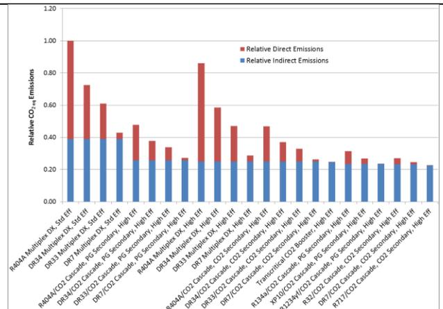
**Figure 4:** Summary of extending relative indirect and direct emissions for various refrigeration products by (Fricke et al, 2013) to more potential refrigerant options
