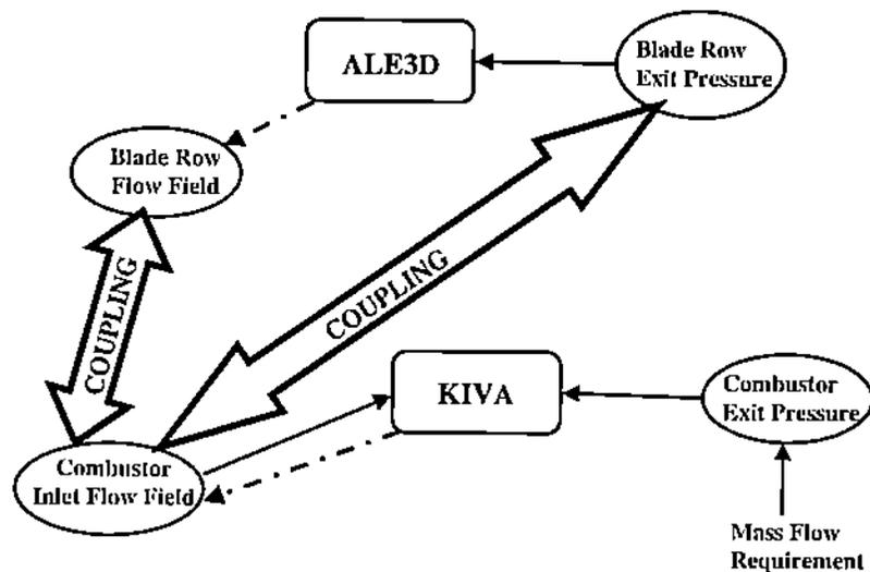
Figure 8. Coupled gas turbine engine transient simulation schematic
