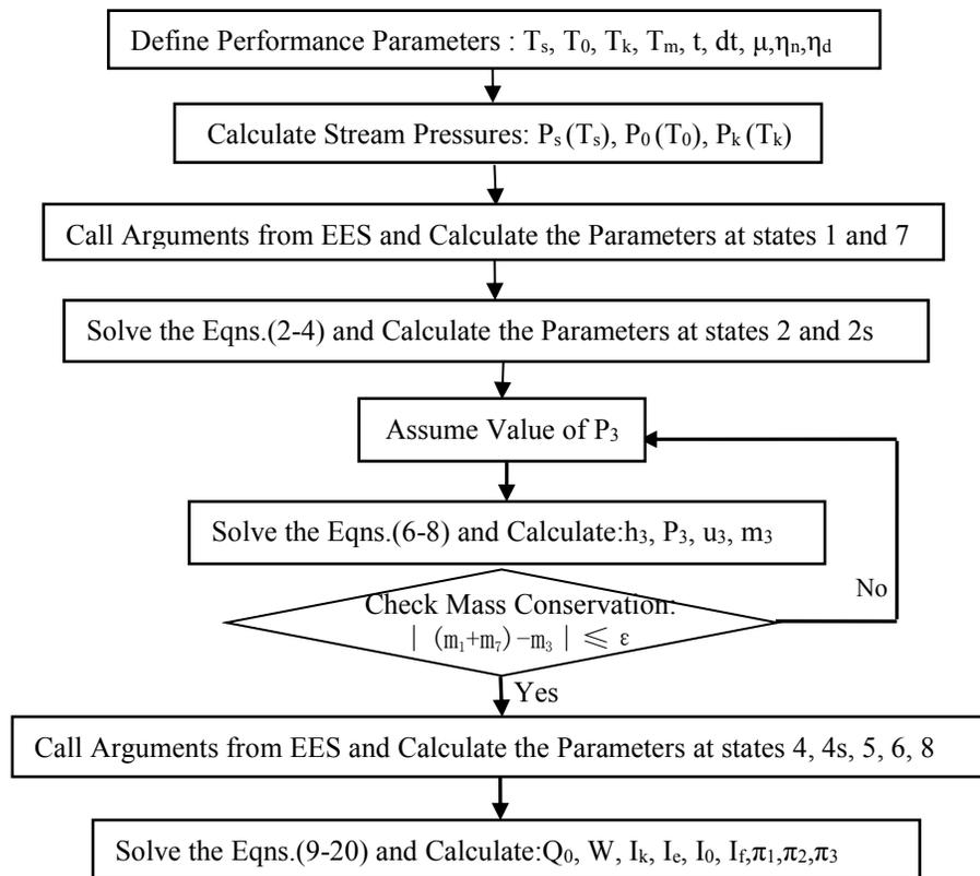
**Figure 3:** Solution algorithms of the iterative process
