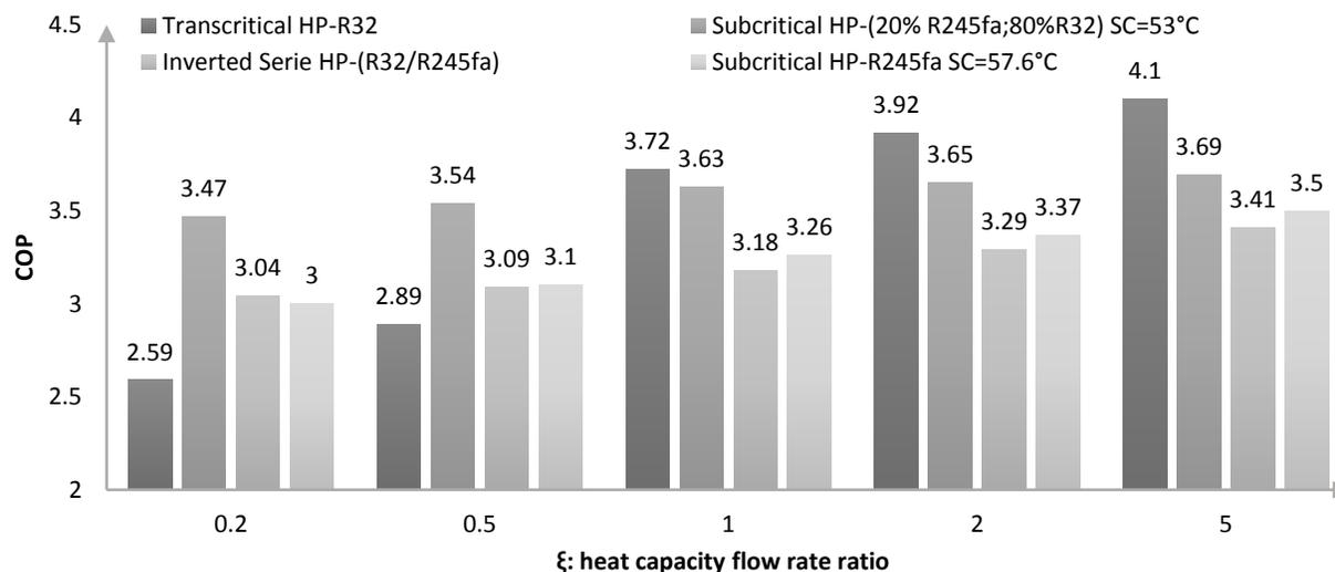
**Figure 5:** Optimal results in term of COP, for heat pumps with  $\Delta T_{SC}$  optimized for all subcritical cycles,  $\Delta T_{SH} = 5^\circ\text{C}$  for all cycles and the high supercritical pressure optimized for the transcritical cycle.
