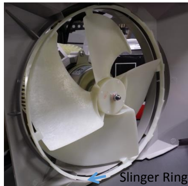
Figure 4: Slinger on condenser fan
