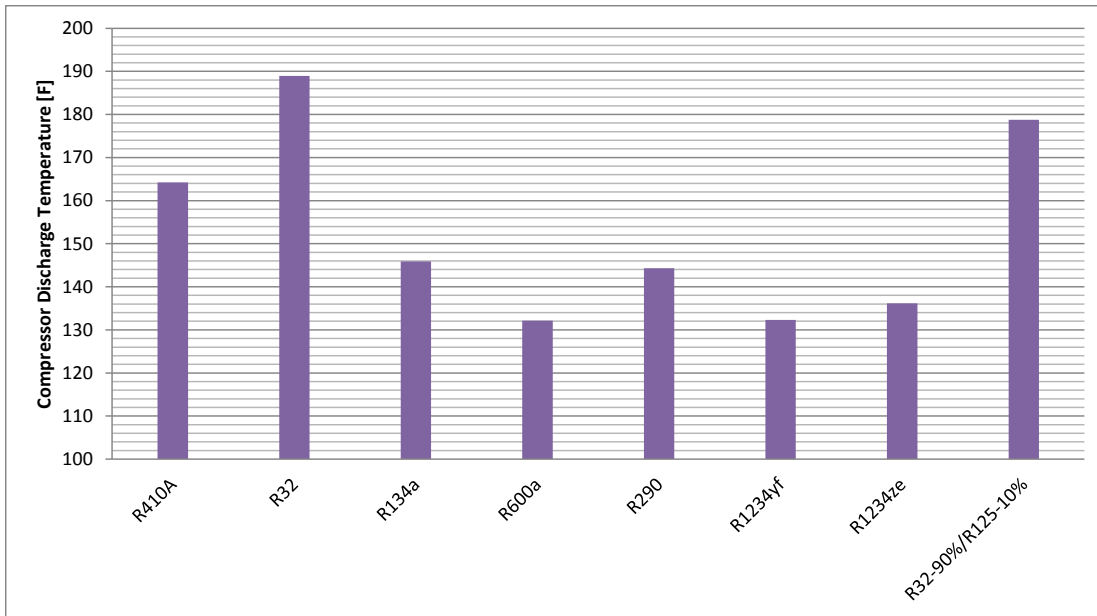
Figure 12: Compressor Discharge Temperatures of Various Refrigerants
