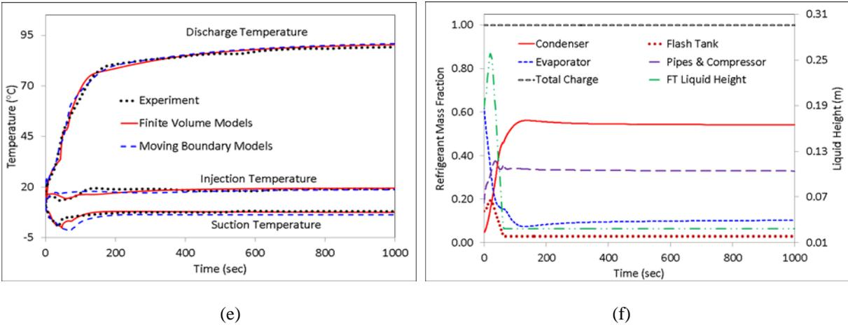
**Figure 4:** Start-up transients: (a) pressure response; (b) condenser heat load response; (c) suction superheat response; (d) injection superheat response; (e) temperature response; (f) simulated refrigerant charge distribution and liquid height in flash tank
