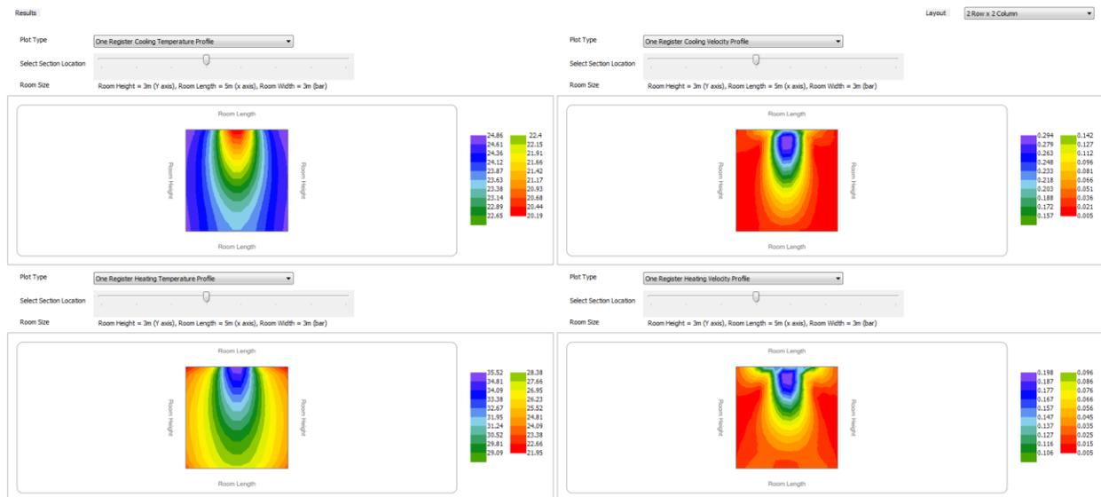
**Figure 7:** Sample POD results of temperature and velocity profile for the mid-plane (left top: temperature profile during cooling; right top: velocity profile during cooling; left bottom: temperature profile during heating; right bottom: velocity profile during heating)
