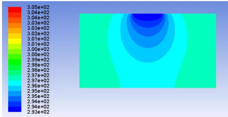
**Figure 4:** Air temperature (in K) profile of one induced-air supply unit (cooling case, middle plane)
