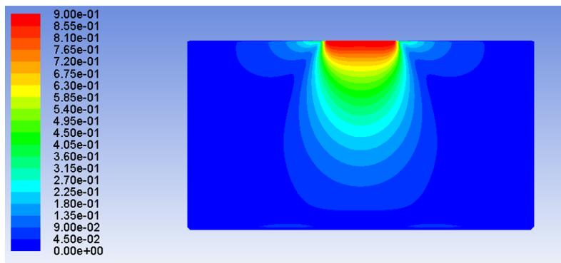
**Figure 5:** Air velocity (in m/s) profile of one induced-air supply unit (heating case, middle plane)
