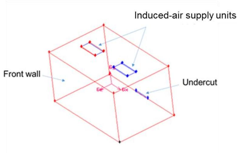
**Figure 2:** Computational domain for a room with two induced-air supply units
