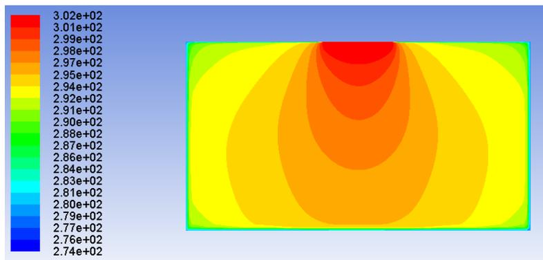
**Figure 6:** Air temperature (in K) profile of one induced-air supply unit (heating case, middle plane)
