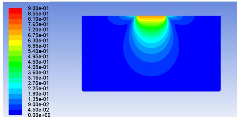
**Figure 3:** Air velocity (in m/s) profile of one induced-air supply unit (cooling case, middle plane)
