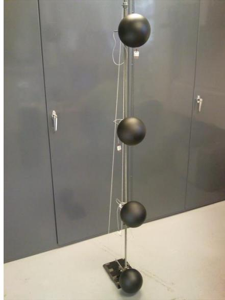
**Figure 11:** Sample of thermocouples on the pole (when mean radiation temperature measurement is not required, black spheres may be removed and the inside thermocouples may be exposed)
