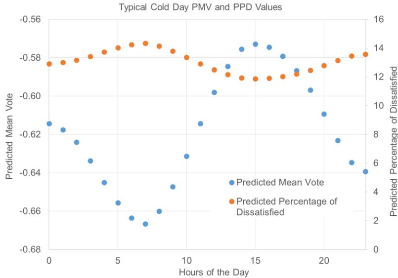
**Figure 10:** Predicted PMV and PPD for a typical cold day
