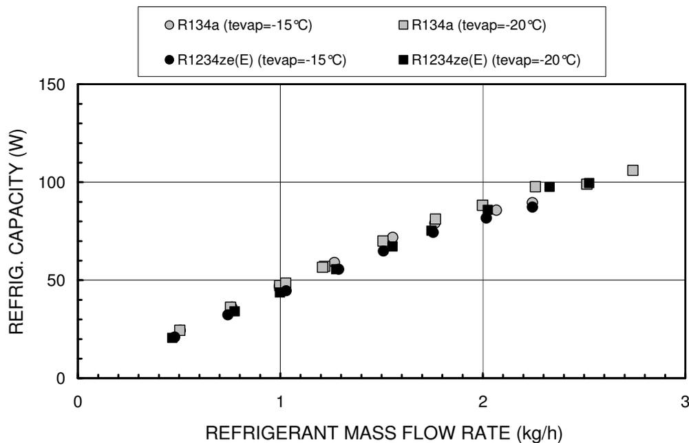
**Figure 4:** Refrigerant capacity vs. refrigerant mass flow rate
