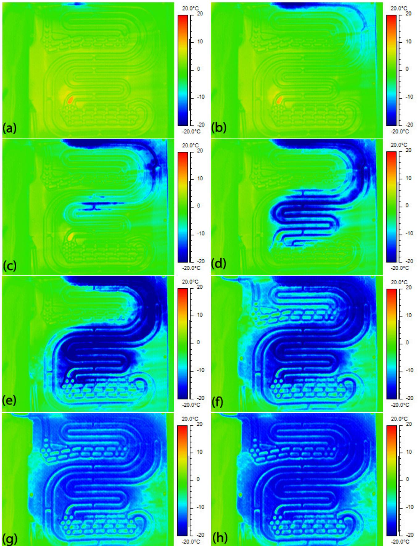
**Figure 3:** Roll bond images collected by the thermal camera. Data with R134a at  $t_{\text{evap}} = -15^\circ\text{C}$ .
