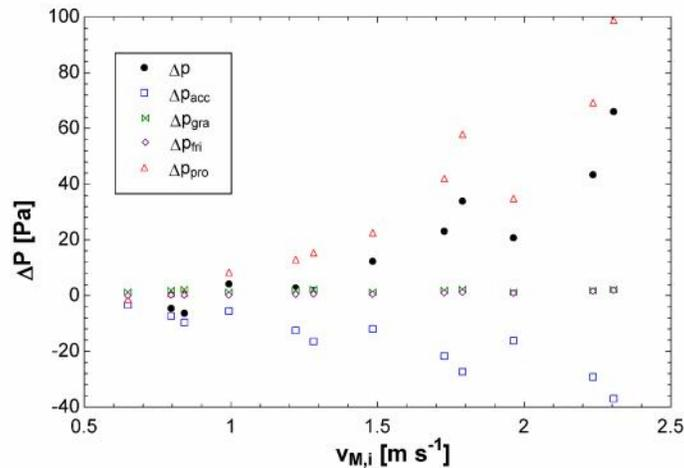
Figure 5: Overall, acceleration, gravitation, friction, and minor pressure drops (R134a vapor)
