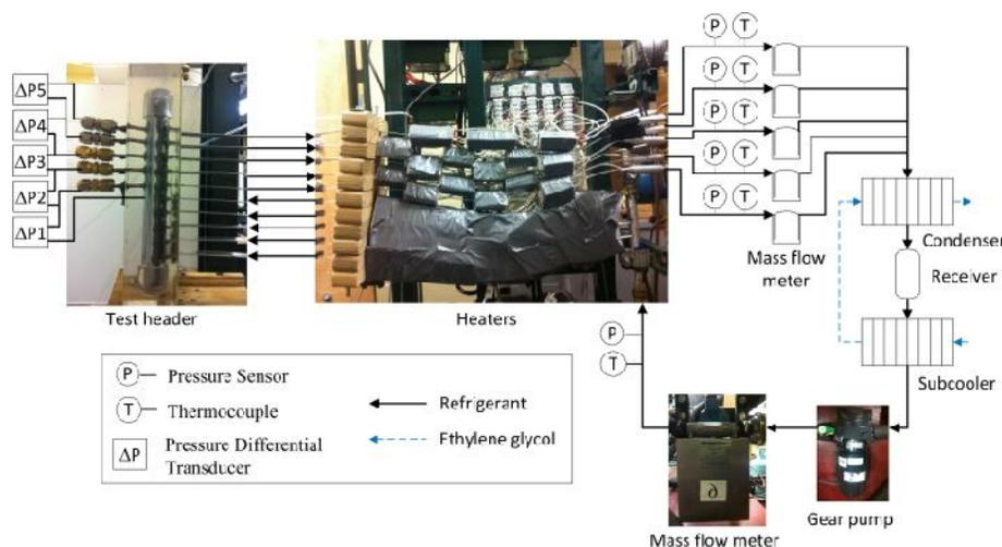
**Figure 1:** System schematics
