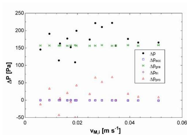
**Figure 9:** Overall, acceleration, gravitation, friction and, minor pressure drops (R134a liquid)
