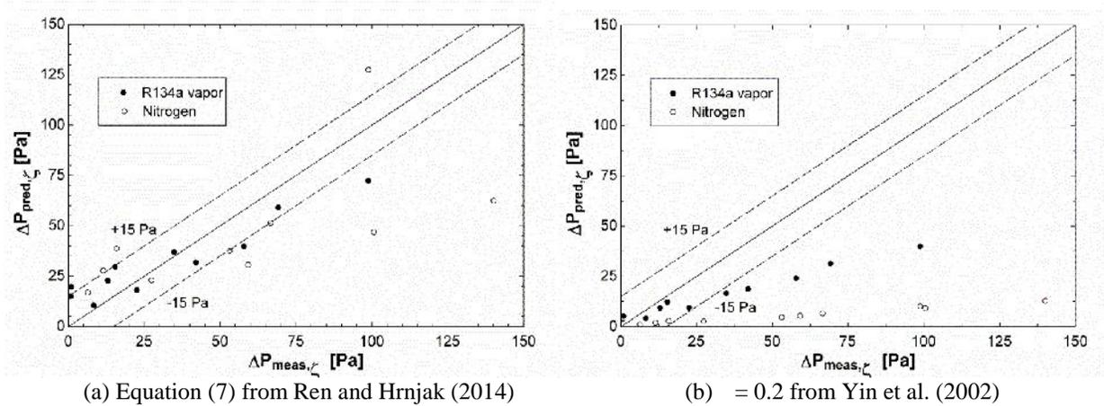
**Figure 7:** The predicted minor pressure drop vs. the measured minor pressure drop (nitrogen and R134a vapor)
