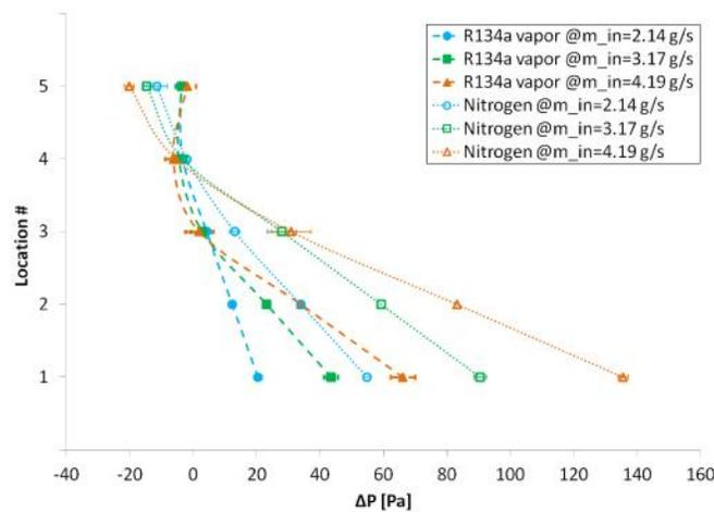
**Figure 3:** Local pressure drop in the header (nitrogen and R134a vapor)
