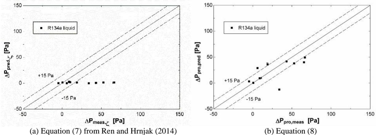
**Figure 10:** The predicted minor pressure drop vs. the measured minor pressure drop (R134a liquid)
