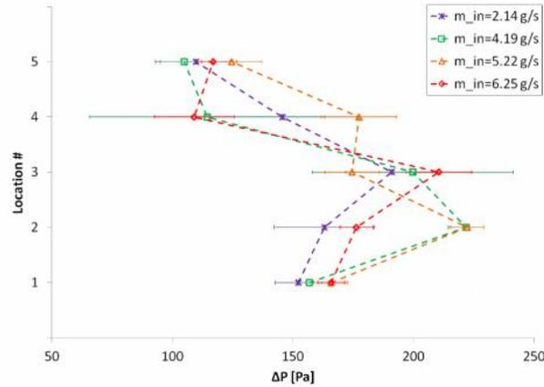
**Figure 9:** Local pressure drop in the header (R134a liquid)
