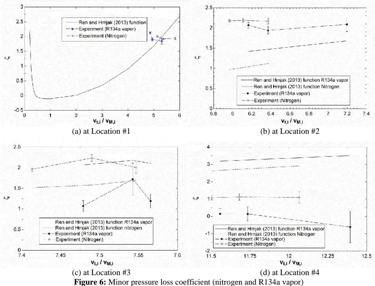
Figure 6: Minor pressure loss coefficient (nitrogen and R134a vapor)
