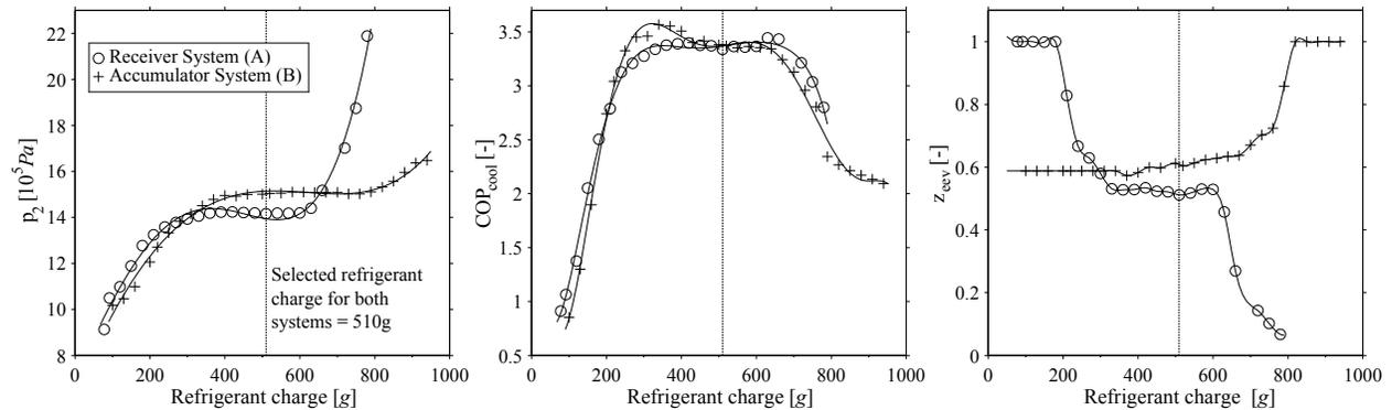
**Figure 4:** Comparison of high pressure  $p_2$ ,  $COP_{cool}$  and relative valve opening  $z_{eev}$  of both systems for increasing overall refrigeration charge. The chosen charge is marked near the center of the high pressure and  $COP_{cool}$  plateau.
