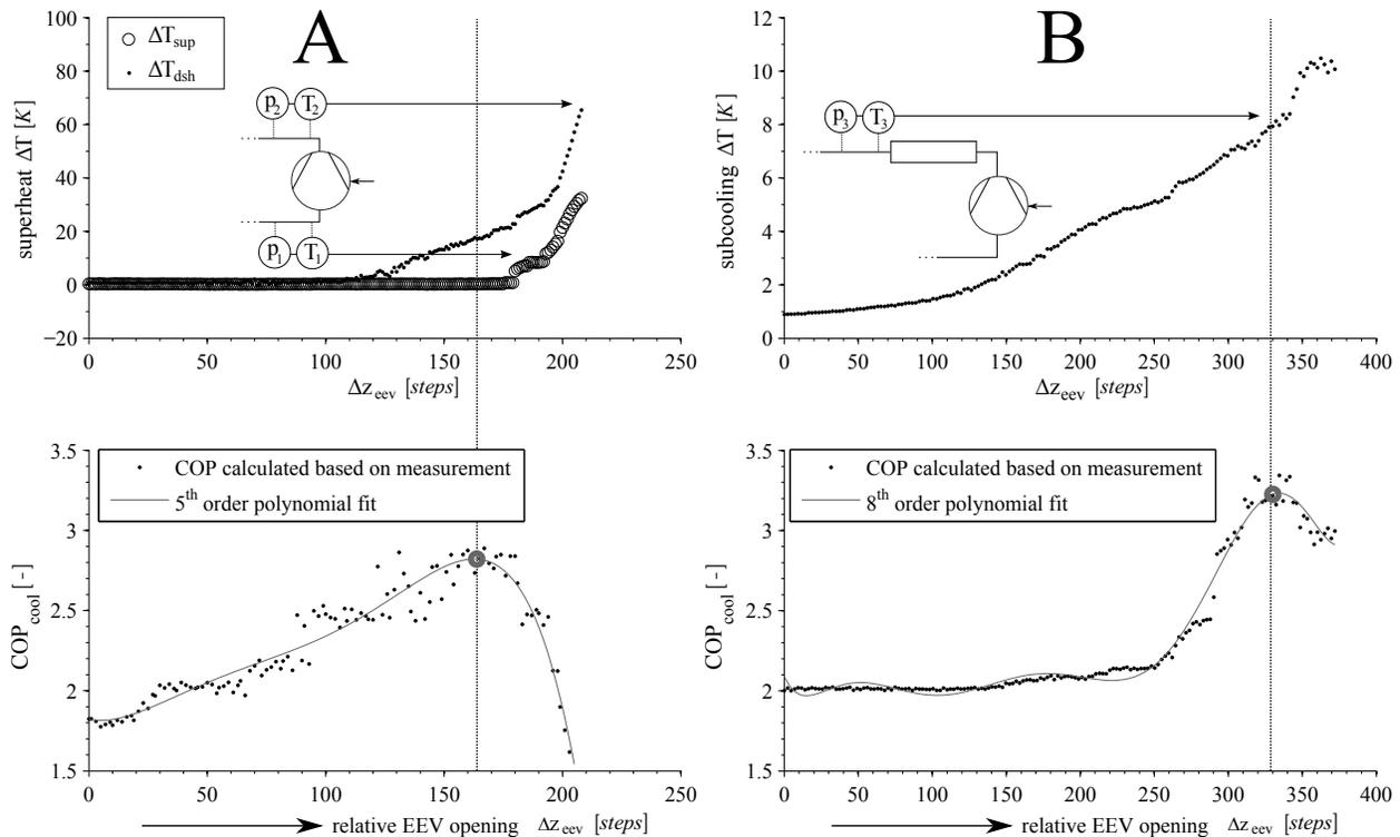
**Figure 5:** Left: Superheating and energy efficiency ( $COP_{cool}$ ) for the receiver system (A). Right: Subcooling and energy efficiency ( $COP_{cool}$ ) for the accumulator system (B). The EEV is closed at very slow speed with a 1% change of the opening every 72 minutes (A) / 10 minutes (B) keeping inflow temperatures ( $T_e = 5^\circ C$ ,  $T_c = 27^\circ C$ ), coolant mass flow rates (both 0.1 kg/s) and cooling power ( $\dot{Q}_{cool} = 1000W$ ) constant (reheat case).
