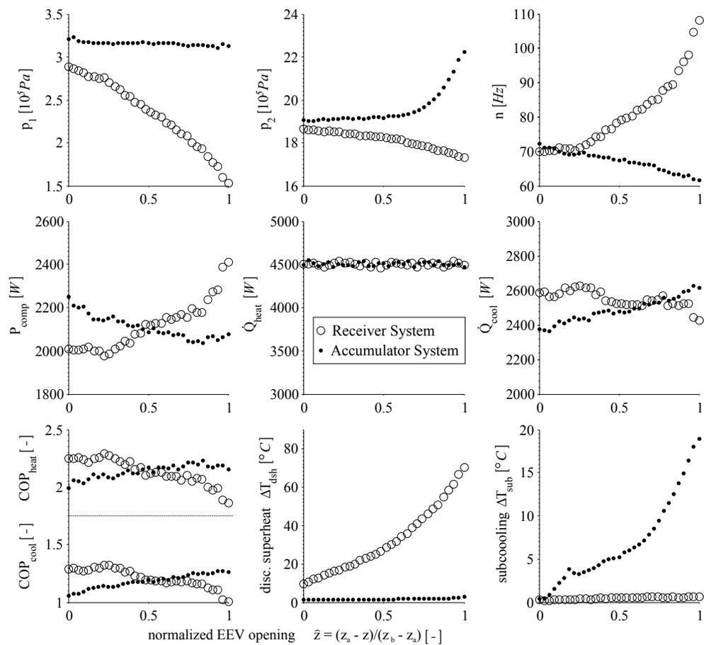
**Figure 7:** System with high pressure receiver compared to a system with low pressure accumulator at the same operating point: Inflow temperatures ( $T_e = 25^{\circ}C \pm 0.3^{\circ}C$ ,  $T_c = 52^{\circ}C \pm 0.5^{\circ}C$ ), mass flow rates (both  $0.1 \text{ kg/s} \pm 0.002 \text{ kg/s}$ ) and heat load ( $\dot{Q}_{heat} = 4500W \pm 99W$ ) are kept constant.
