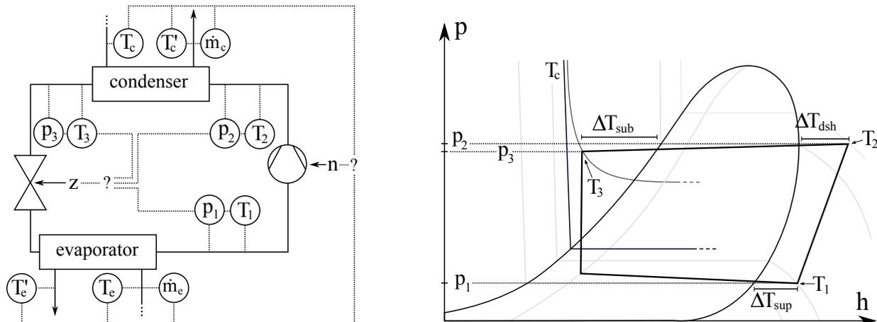
**Figure 2:** Basic control concept: The compressor speed  $n$  is used to fulfill load requirements (cooling power or heating power) while the electronic expansion valve is used either to control superheat  $\Delta T_{sup}$ , discharge superheat  $\Delta T_{dsh}$  or subcooling  $\Delta T_{sub}$  depending on the system configuration
