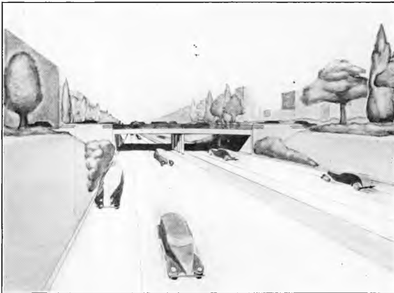
Fig. 3. Sketch of type of depressed highway construction considered for the Clybourn-Elston Route and the Bryn Mawr-River-Clybourn Route.
