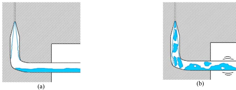
Figure 6: Illustration of the flow pattern at the evaporator inlet as a consequence of vapor (a) and slug (b) flow at the entrance of the capillary.
