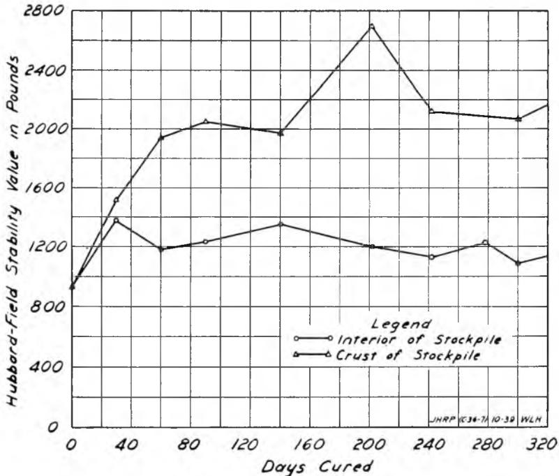
Fig. 2. Effect of stockpile curing on Hubbard-Field stability values of soft rock asphalt.
