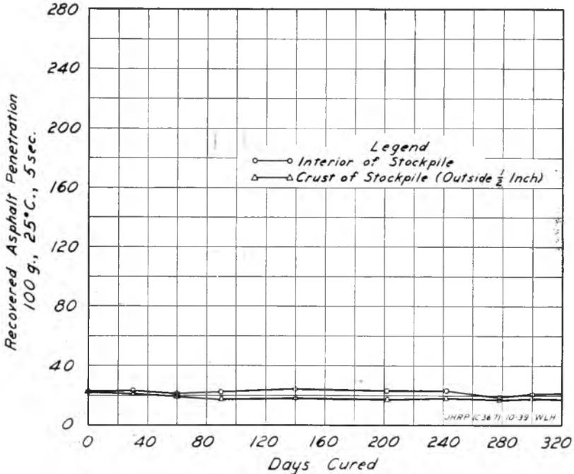
Fig. 3. Effect of stockpile curing on penetration of hard asphaltic sandstone.
