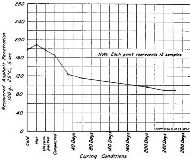
Fig. 6. Composite chart showing effect of road curing on penetration of soft rock asphalt in three roads.
