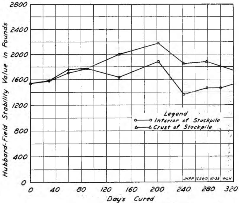
Fig. 4. Effect of stockpile curing on Hubbard-Field stability values of hard rock asphalt.
