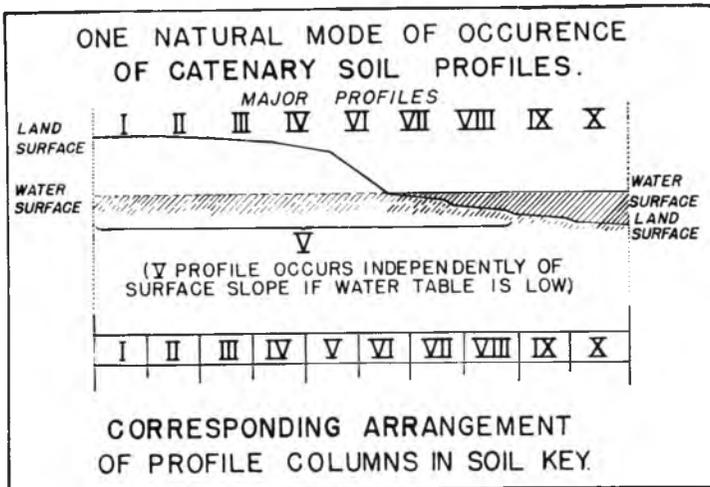
Fig. 5. Illustrating effects of water relationship on soil classification.
