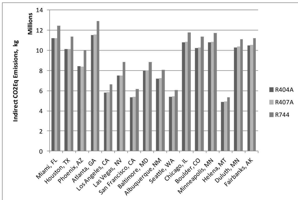
**Figure 6:** Lifetime Indirect Emissions due to Supermarket Refrigeration System Operation
