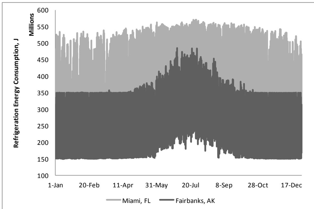
**Figure 3:** R404A Refrigeration system energy consumption over a year in weather extremes: Miami, FL and Fairbanks, AK with an average energy consumption of 396 MJ and 254 MJ respectively.
