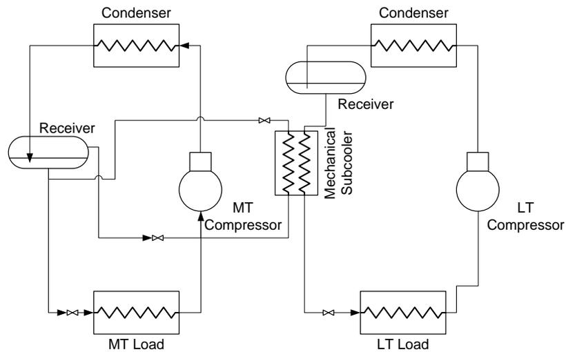
Figure 1: Typical multiplex DX system configuration
