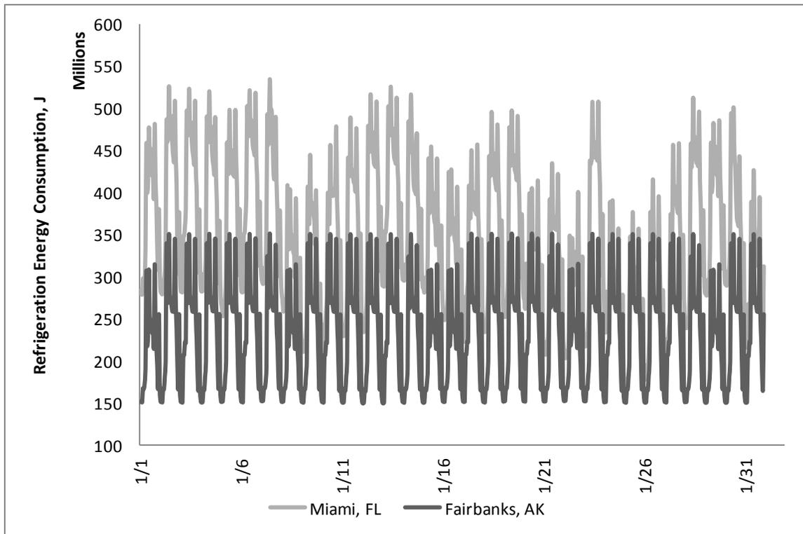
**Figure 4:** R404A Refrigeration system energy consumption for the month of January in weather extremes: Miami, FL and Fairbanks, AK with an average energy consumption of 348 MJ and 232 MJ respectively.
