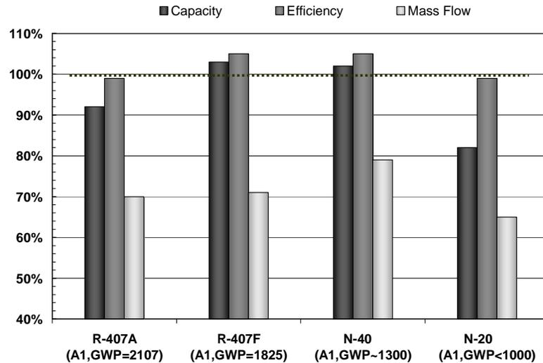
Figure 3. Medium Temperature Tests (relative to R-404A).
