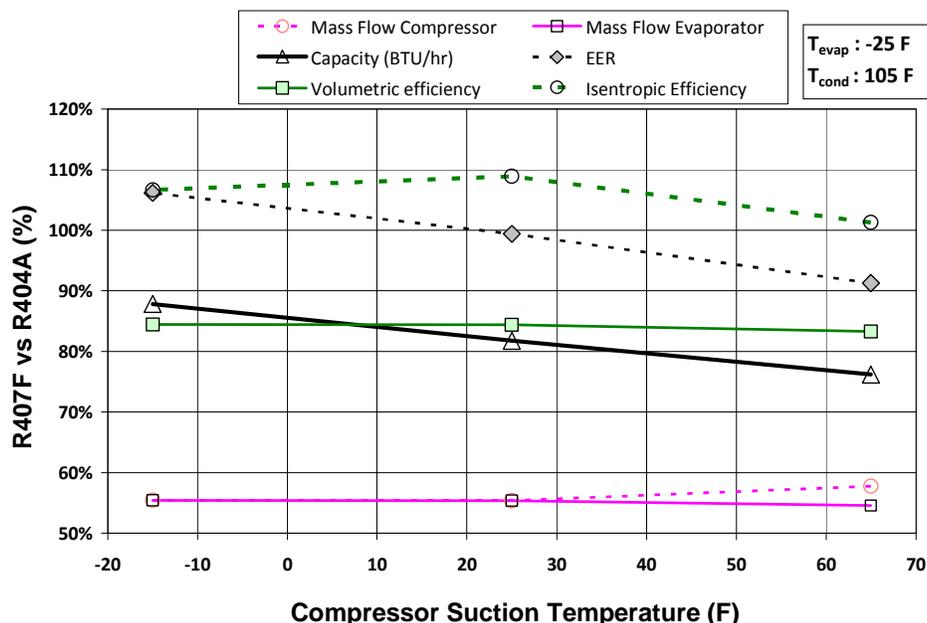
Figure 8. Effect of suction temperature on compressor efficiency.
