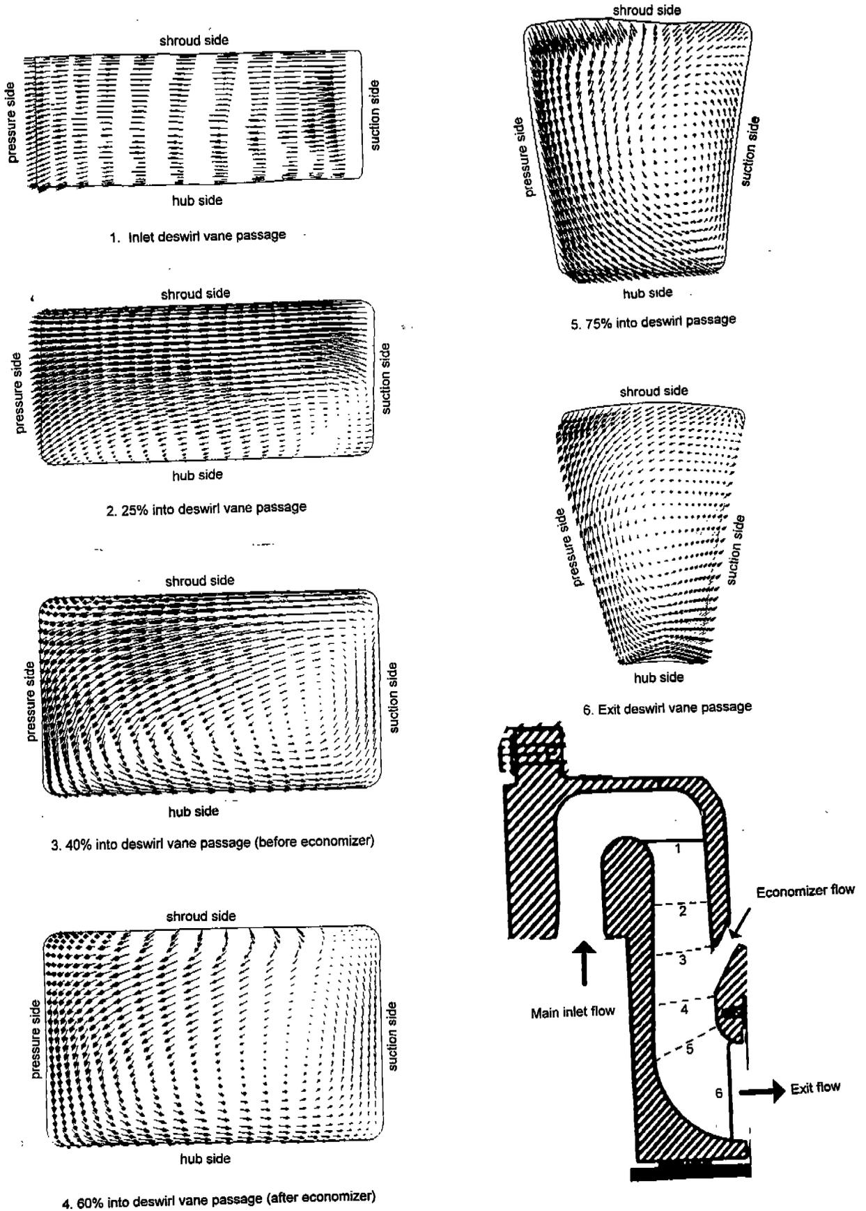
*Figure 7. Velocity projections in six circumferential planes normal to the throughflow direction between inlet and exit of the deswirl vane section of the return channel.*
