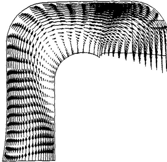
Figure 5. Meridional projection of velocities in the vaneless diffuser and the cross-over bend
