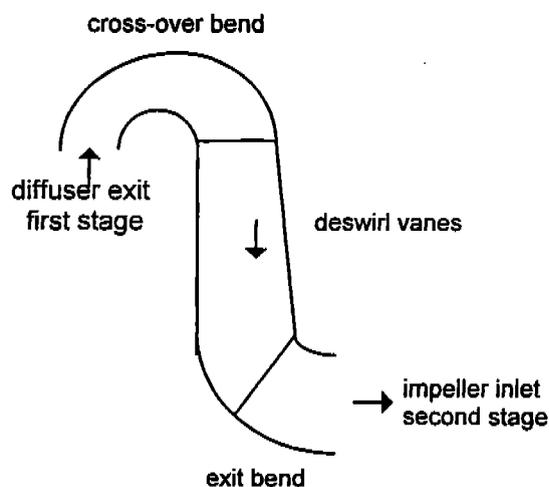
Figure 1. Return channel geometry definition
