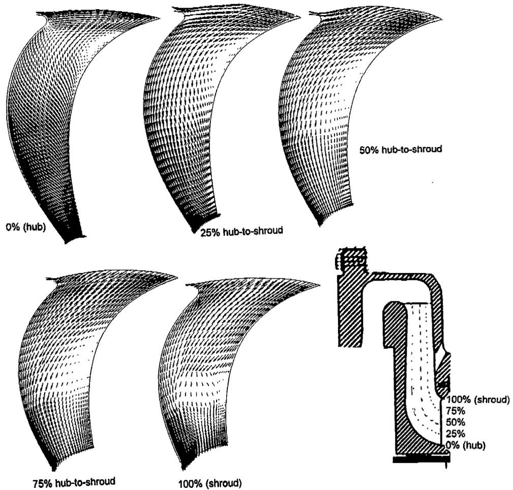
Figure 6. Velocity plots in the circumferential (blade-to-blade) plane at various hub-to-shroud locations
