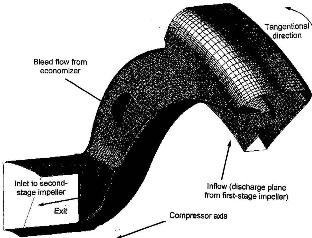
*Figure 4. Computational grid for the return channel of the 2,000 ton HFC-134a compressor.*
