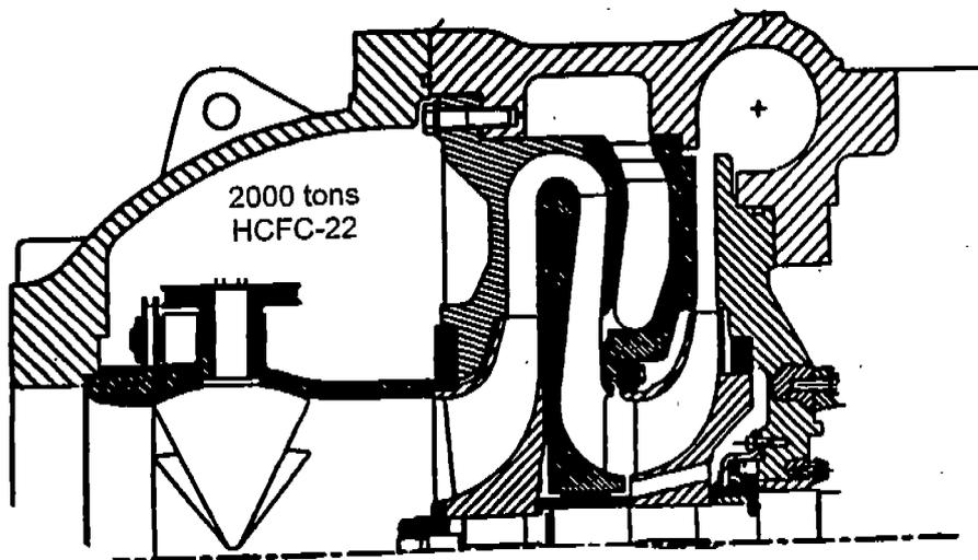
Figure 2. Cross-section of 2000 ton two-stage centrifugal compressor using HCFC-22
