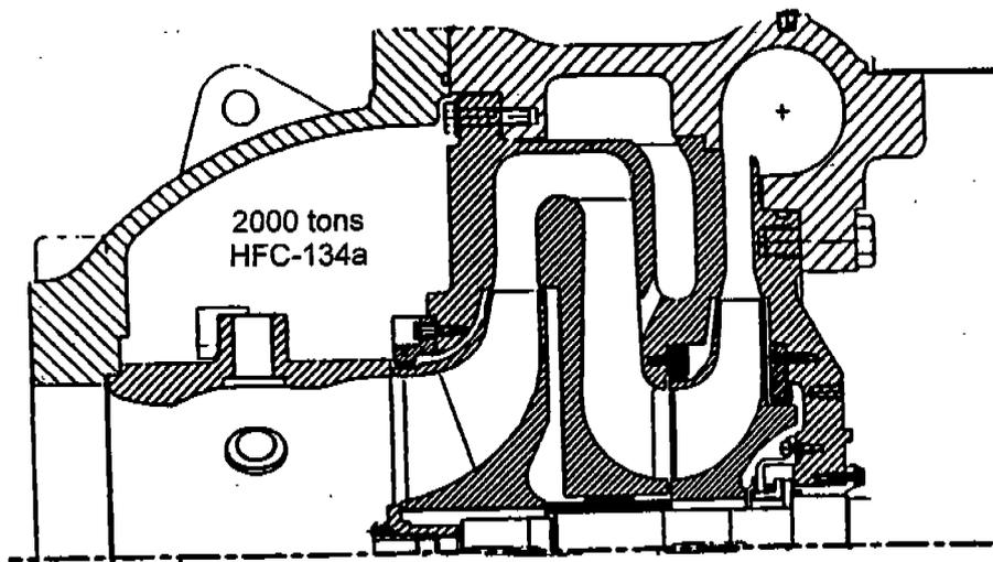
Figure 3. Cross-section of redesigned 2000 ton two-stage centrifugal compressor using HFC-134a
